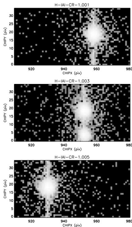
Figure 1: Images constructed from telemetry event lists for XRCF tests H-IAI-CR-1.001, 1.003, and 1.005 (top to bottom). From the top to the bottom panel, source flux increases by about an order of magnitude.
