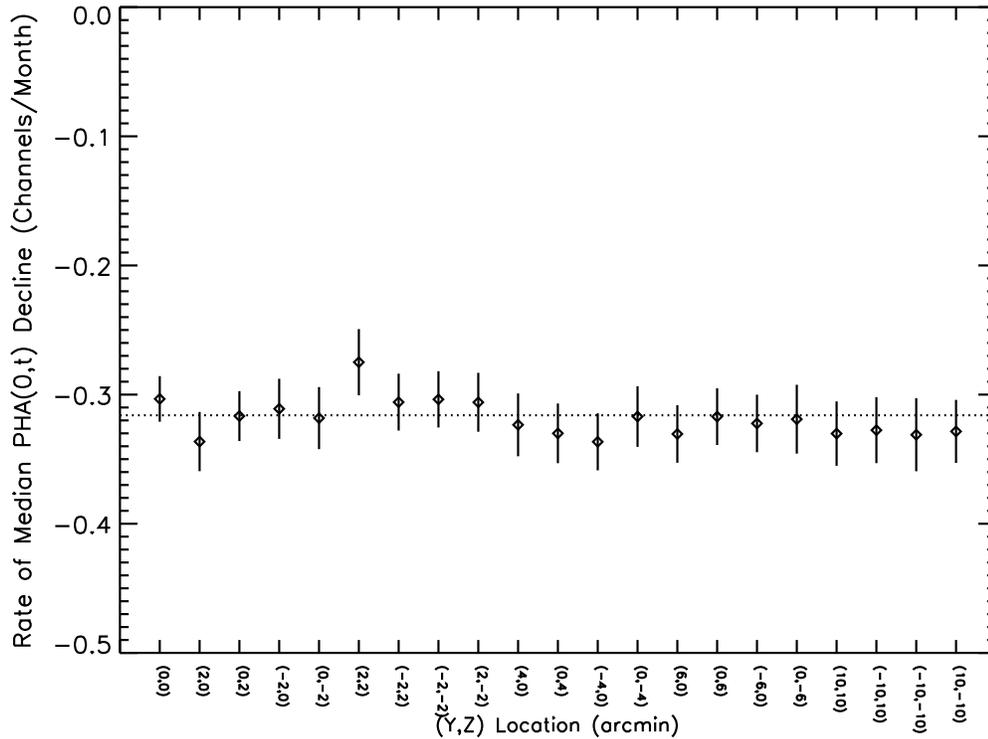
Figure 9: Best-fit slopes (with  $1\sigma$  errors) from linear fits to the median spatially-corrected PHAs (excluding Oct and Dec 99) for each observation location. The horizontal dashed line shows the average rate of decline.
