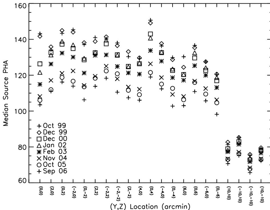
Figure 2: Median PHAs for HRC-I AR Lac observations. The background subtracted median PHAs are plotted in a vertical row for all observations at a given location, for data obtained during different cycles, all at the low voltage setting. Data from different cycles are marked with different point types (see legend). The statistical errors on the medians are typically  $\leq 1$  channel. Note that the median PHAs drop monotonically.
