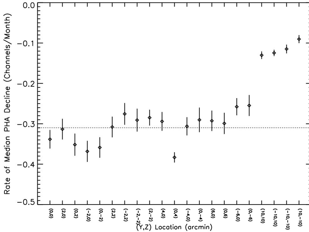
Figure 4: Uniformity of gain decline across the HRC-I. The best-fit slopes from the linear fits to the median PHAs (Figure 3) are shown for each location. The average of the slopes (neglecting the four pointings at 14.14' offaxis) is shown as the dotted horizontal line. To a first approximation, excluding the far offaxis locations, the gain decline is uniform across the detector.
