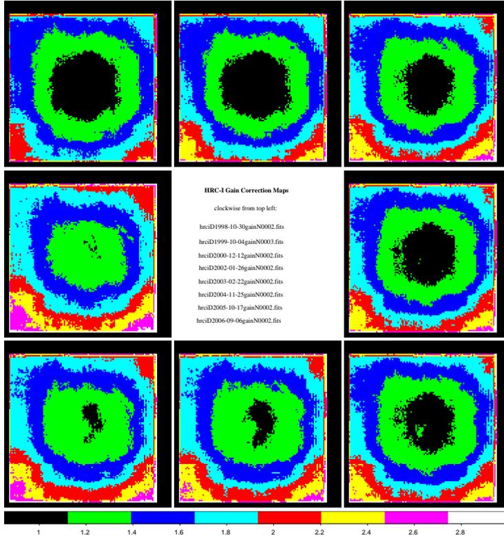
Figure 10: Gain correction maps, shown on a linear display scale from 0.85-3. The pre-flight gain correction map  $g_{\text{LAB}}(\vec{x})$  is in the upper left corner. The subsequent time-dependent maps, with updates based on AR Lac observations, are shown chronologically in clockwise order.
