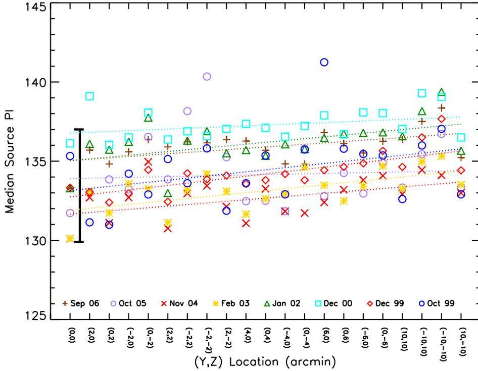
Figure 11: Median PI values of AR Lac datasets, calculated using the new gain correction maps, as a function of observation location. The bold vertical bar at the left shows the typical  $\pm 1\sigma$  error on the medians, which includes the uncertainties in  $\gamma$  and  $TC(t)$ , typically  $\sim 1\%$  and  $\sim 2\%$ , respectively. The horizontal dotted lines show linear least-squares fits to data for each AO. The slopes are statistically consistent with zero.
