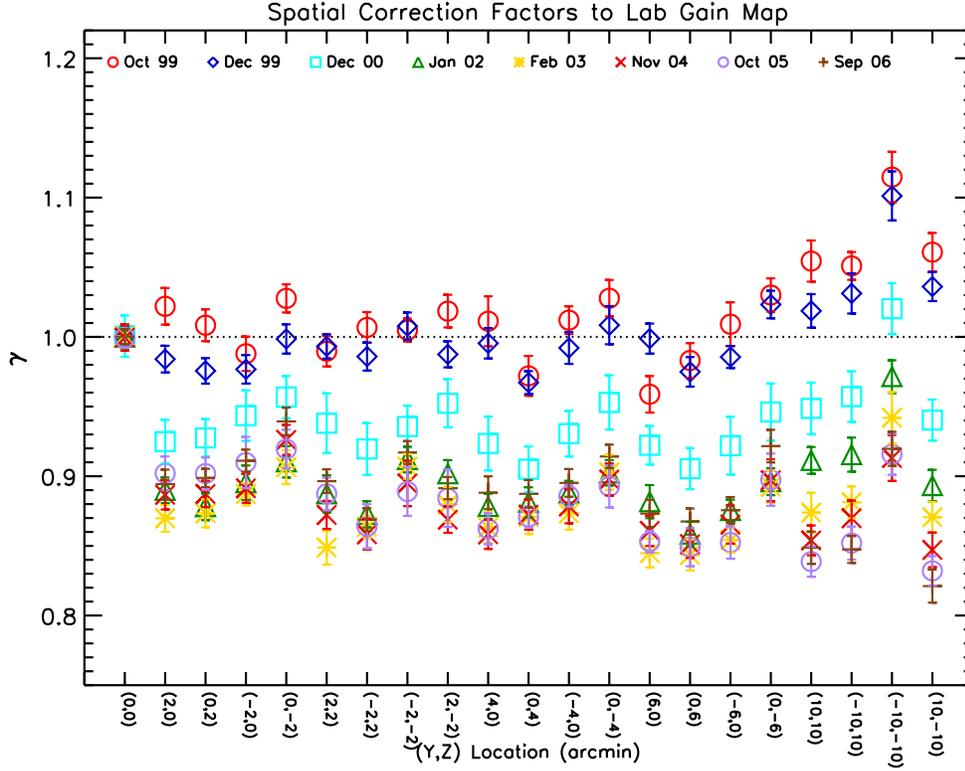
Figure 7: Gain correction factors  $\gamma$  as a function of location on the detector. These correction factors are relative to the pre-flight gain map  $g_{\text{LAB}}(\vec{x})$ .
