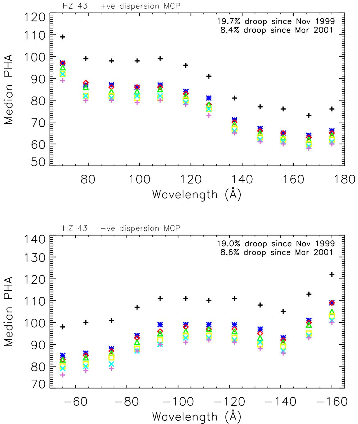
**Figure 5.** HZ 43 median PHA evolution for the 12 dispersion bins on each of the wing MCPs. Top plot: positive dispersion MCP. Bottom plot: negative dispersion MCP.
