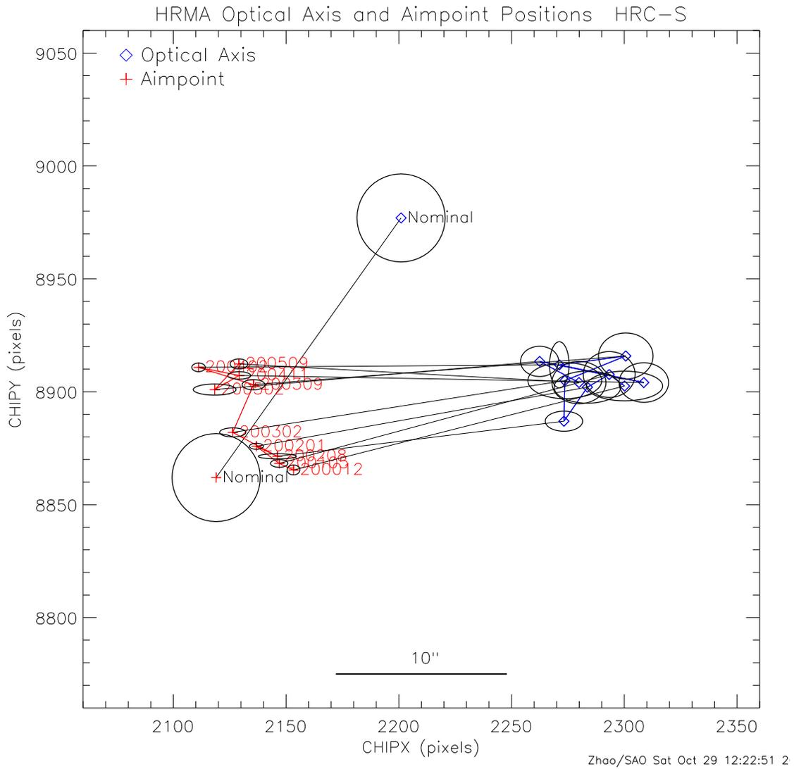
Figure 11: Optical Axis and Aimpoint positions from all the HRC-S measurements on CHIP coordinates.
