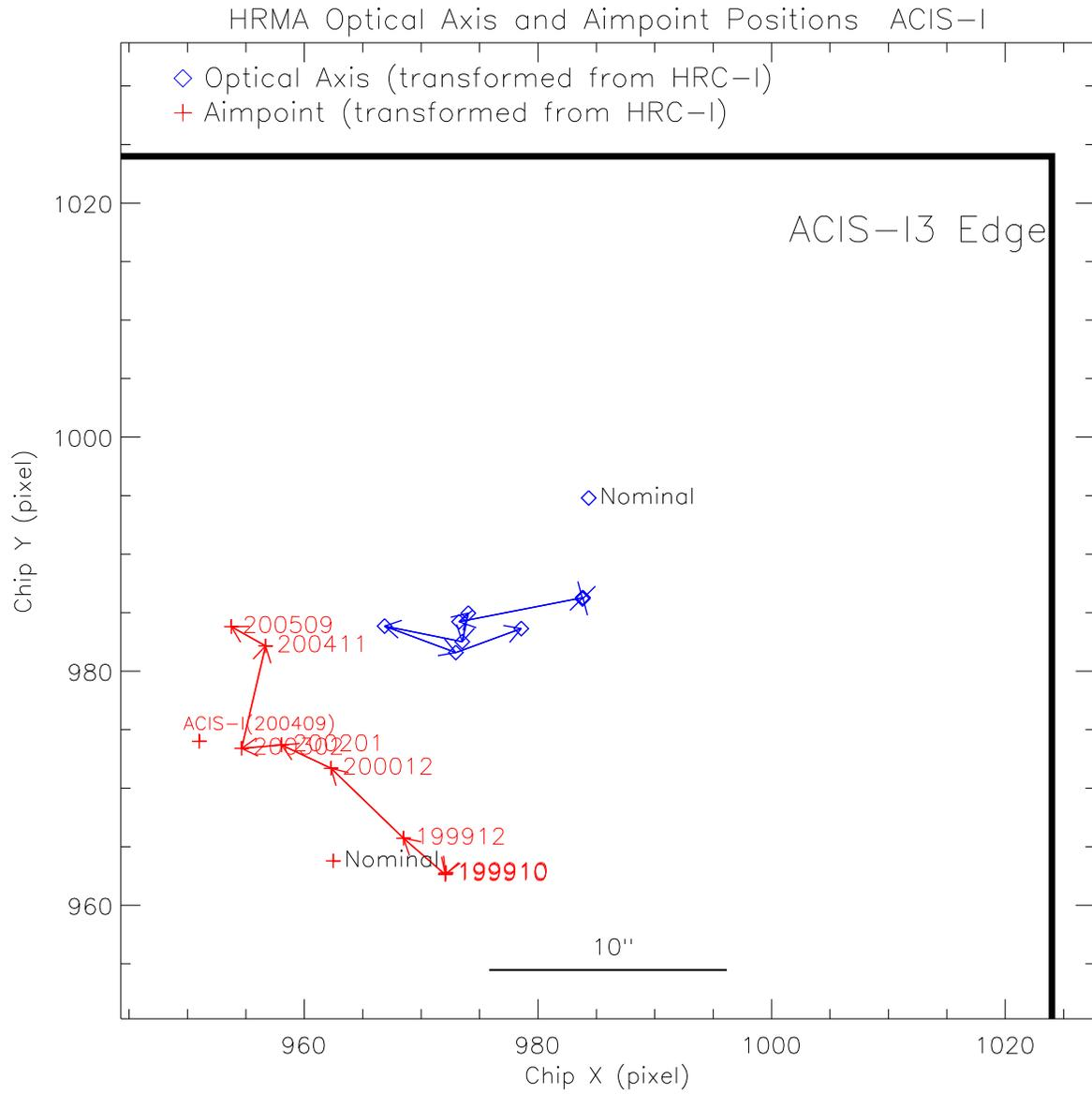
Figure 17: Chandra Optical Axis and Aimpoint positions on ACIS-I, transformed from the HRC-I measurements. (Node boundary is outside of the figure.)
