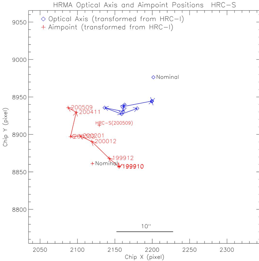
Figure 13: Chandra Optical Axis and Aimpoint position drift on HRC-S, transformed from the HRC-I measurements.
