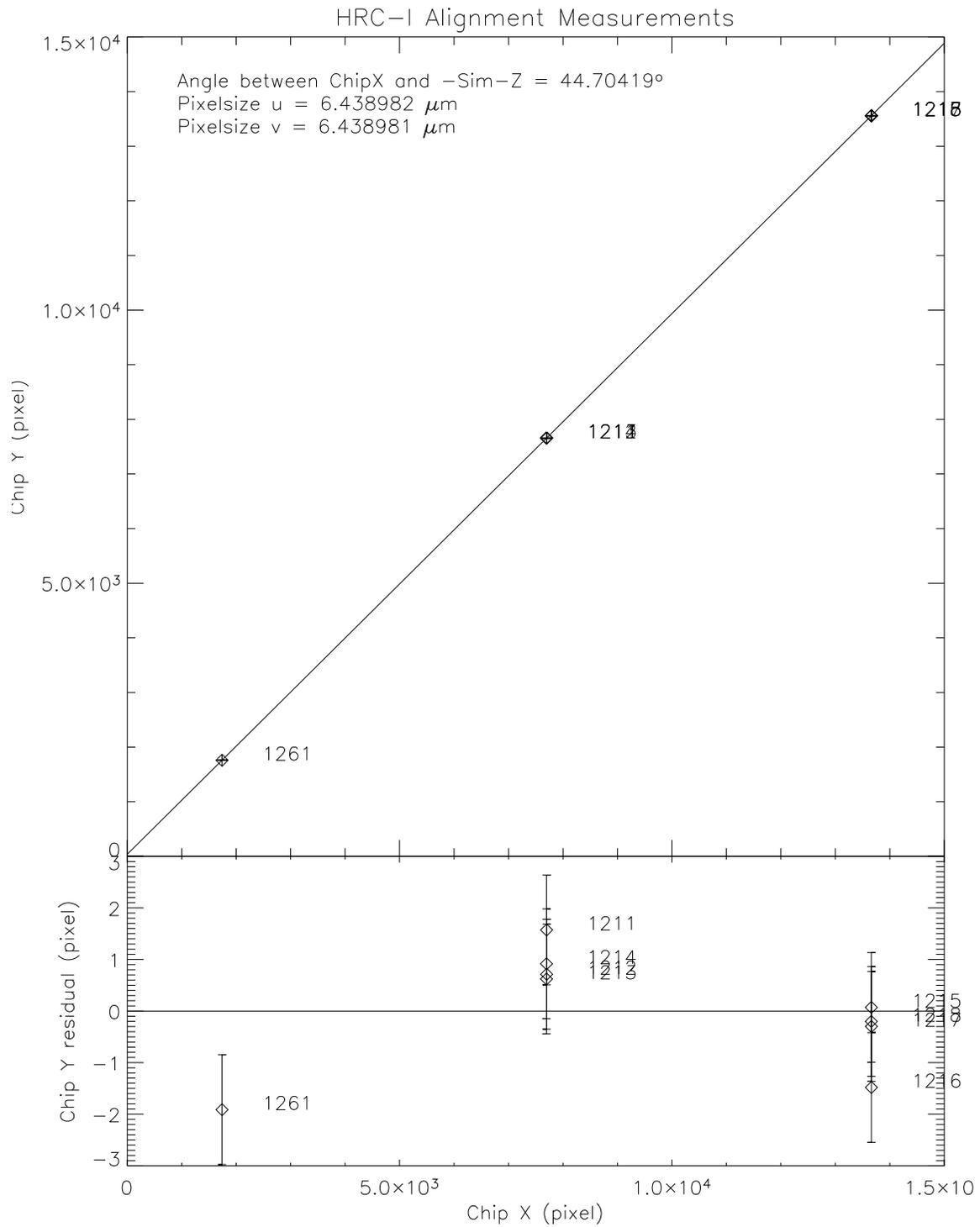
Figure 9: HRC-I alignment measurements (observations with dithering off): results show the clocking angle between +CHIPX and -Sim-Z is  $44.70419^\circ$ , instead of  $45^\circ$ .
