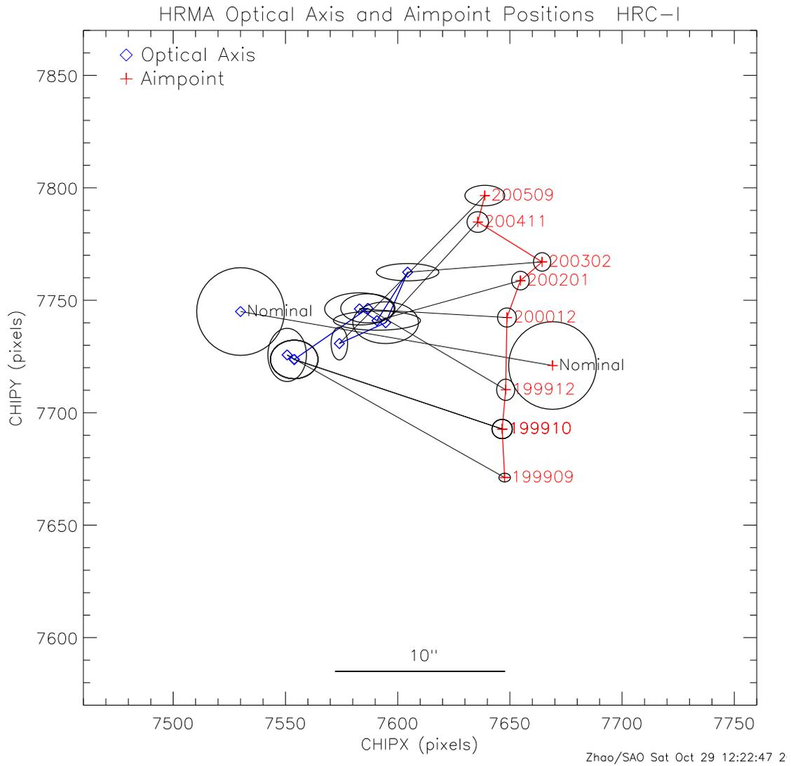
Figure 10: Optical Axis and Aimpoint positions from all the HRC-I measurements on CHIP coordinates.
