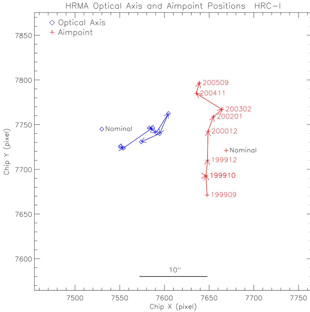
Figure 12: Chandra Optical Axis and Aimpoint position drift on HRC-I.
