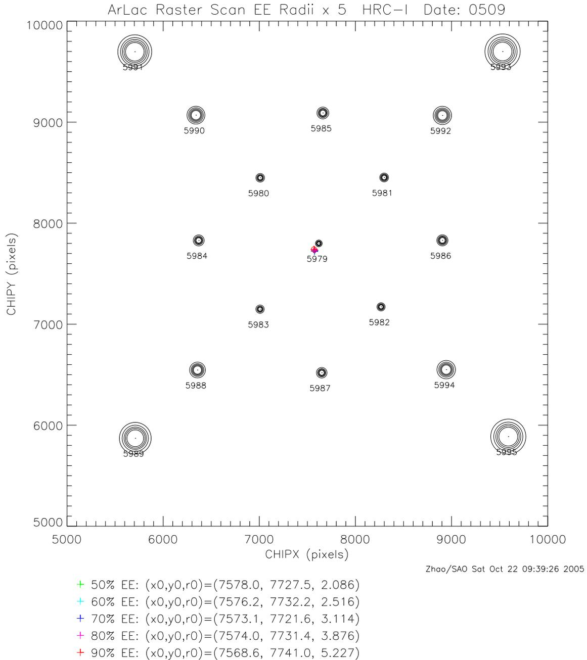
Figure 5: HRC-I raster scan observation of Ar Lac with 1ks exposure time for each scan point (Date: 2005-09-27). Circles around each observation point are the 50% – 90% EE circles  $\times 5$ .
