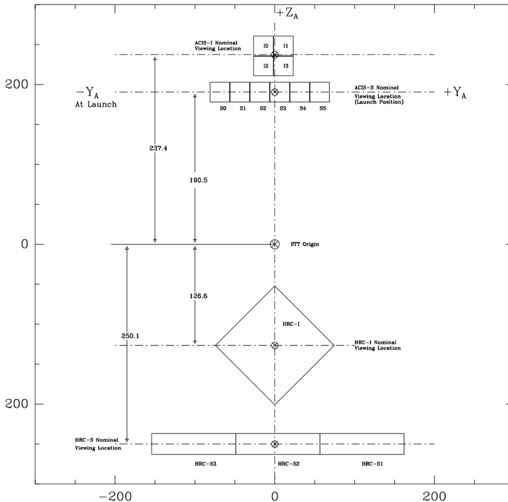
Figure 1: The Chandra SIM Translation Table, showing the flight focal plane instrument to scale. Distance in mm. Coordinate system is AXAF-STT-1.0.
