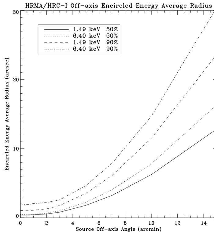
Figure 4.12: HRMA/HRC-I encircled energy average radii for circles enclosing 50% and 90% of the power at 1.49 and 6.40 keV as a function of off-axis angle. The HRC-I surface is a flat plane perpendicular to the optical axis, which does not follow the curved *Chandra* focal plane. These curves include the blurs due to the HRC-I spatial resolution and the *Chandra* aspect error.
