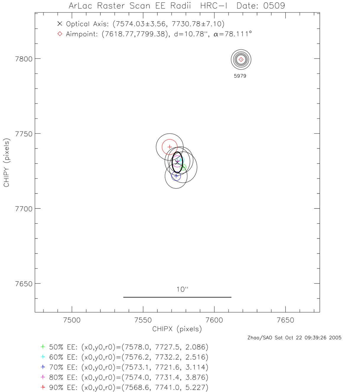
Figure 8: Optical Axis and Aimpoint position on HRC-I, based on raster scan observation of Ar Lac made on 2005-09-27. The center  $\times$  with the dark oval is the optical axis position and its error oval.
