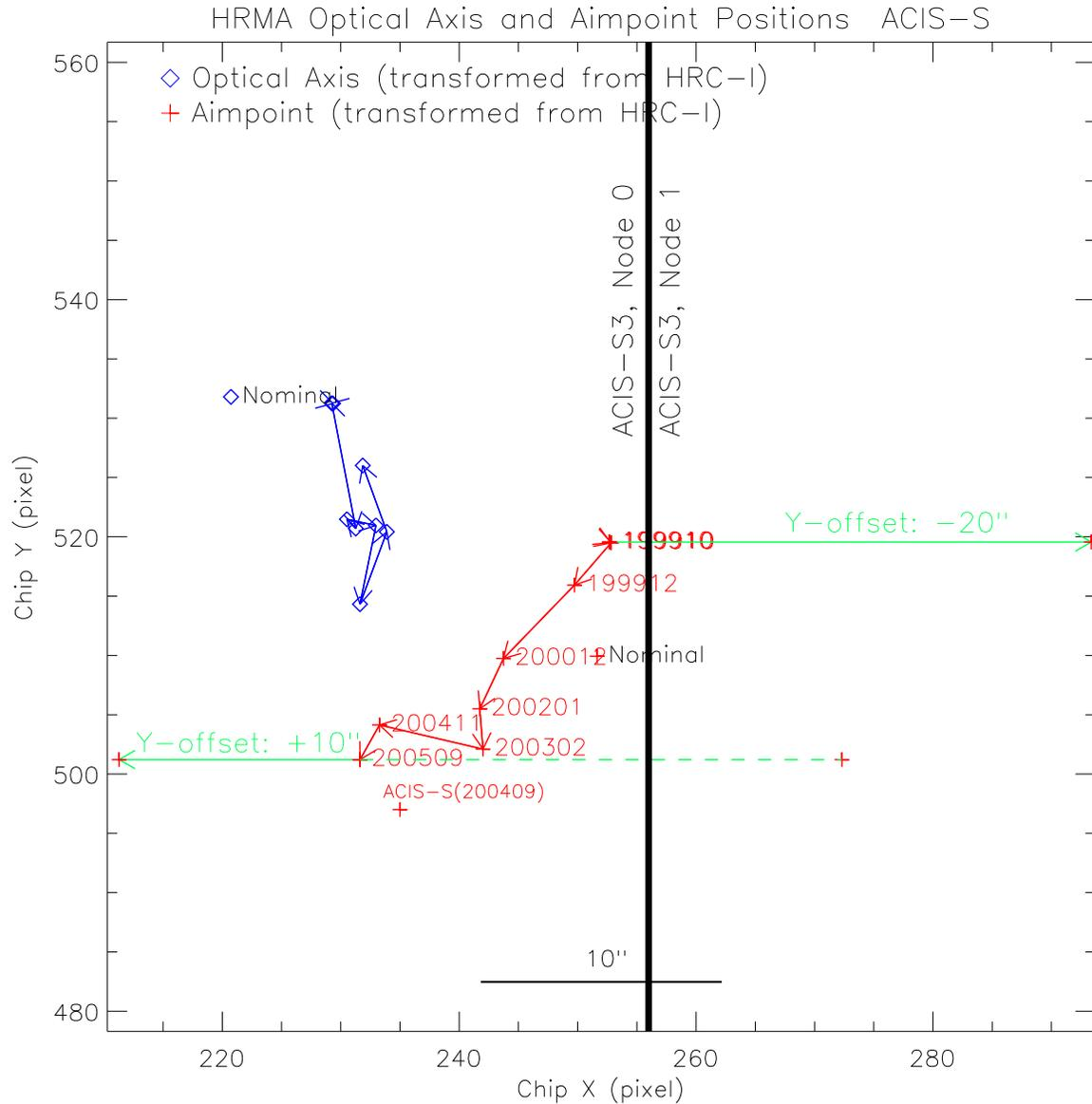
Figure 18: Chandra Optical Axis and Aimpoint positions on ACIS-S, transformed from the HRC-I measurements. Because of the aimpoint drift, the default target pointing offset for ACIS-S observations has been changed from  $Y\text{-offset}=-20''$  to  $Y\text{-offset}+10''$  to avoid the node boundary during dither ( $16''$  peak to peak), as announced in Chandra Electronic Bulletin No. 43. This change also puts the target pointing closer to the Optical Axis.
