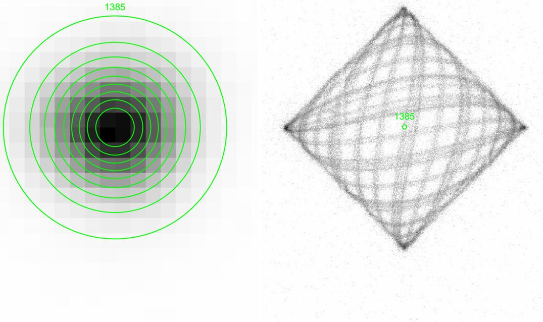
Figure 2: HRC-I observation of Ar Lac with 19ks exposure time and zero Y and Z offsets (obsid 1385). Left: image in SKY coordinates with 10% – 90% encircled energy circle overlay. Right: image in CHIP coordinates with the calculated center marked. This calculated center is at the center of the Lissajous dither pattern.
