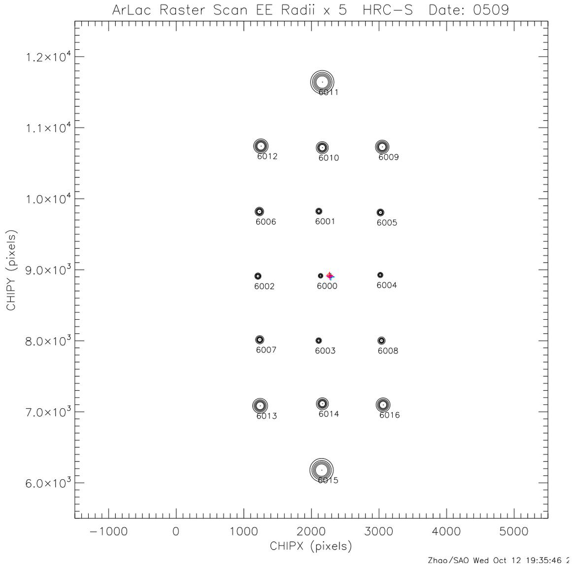
Figure 6: HRC-S raster scan observation of Ar Lac with 1ks exposure time for each scan point (Date: 2005-09-01). Circles around each observation point are the 50% – 90% EE circles  $\times 5$ .
