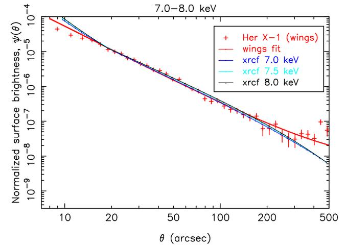
Figure D.4: Powerlaw plus exponential cutoff fits to the obsid 3662 (Her X-1 wings) data; the fits were for  $\theta \geq 15''$ . Mirror vignetting was included in exposure correcting the data (see text). The model based on ground calibration data is also indicated (labeled “xrcf”).
