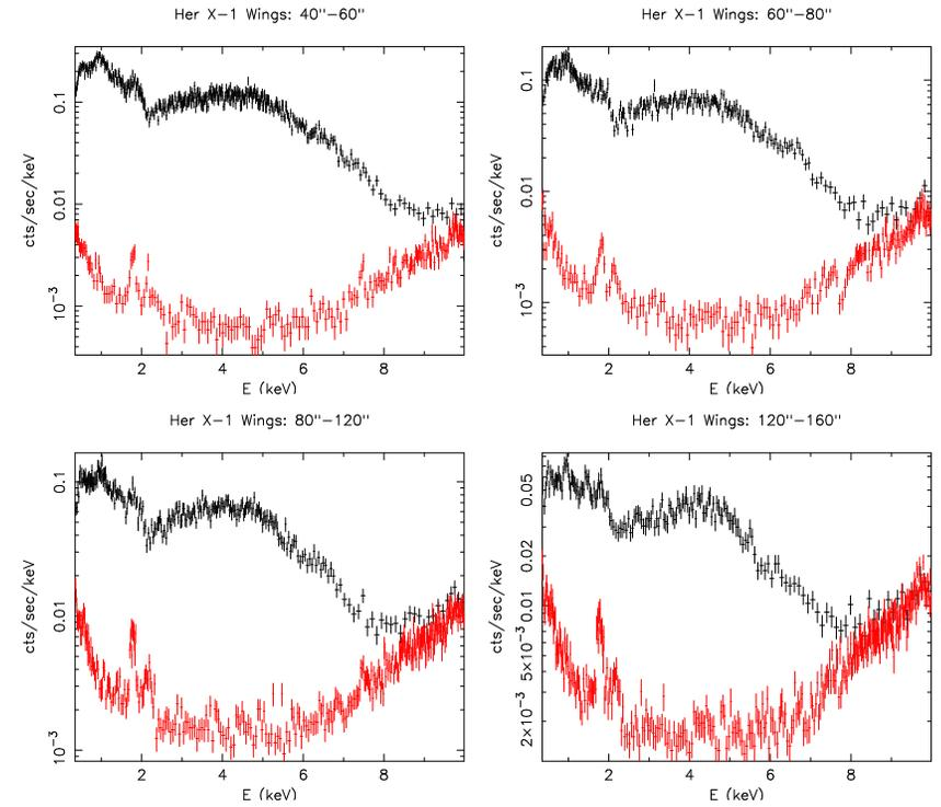
Figure E.3: Spectrum of the Her X-1 diffuse mirror scattering wings (excluding the core ACIS transfer streak). Top Left:  $40'' - 60''$ ; source and blank sky. Top Right:  $60'' - 80''$ ; source and blank sky. Bottom Left:  $80'' - 120''$ ; source and blank sky. Bottom Right:  $120'' - 160''$ ; source and blank sky.
