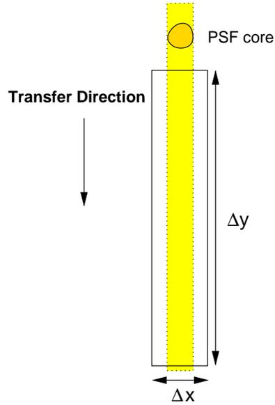
Figure B.1: Schematic of the transfer streak calculation.  $\Delta x$  should be large enough to include the core and near wings, but small enough to minimize the enclosed background.  $\Delta y$  should extend over a region far enough away from the source that the included wing profile is small compared to the transfer streak contribution. A corresponding box on the other side of the direct image can be added to improve the statistics.
