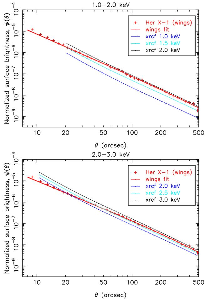
Figure D.1: Powerlaw plus exponential cutoff fits to the obsid 3662 (Her X-1 wings) data; the fits were for  $\theta \geq 15''$ . Mirror vignetting was included in exposure correcting the data (see text). The model based on ground calibration data is also indicated (labeled “xrcf”). Top: 1.0-2.0 keV. Bottom: 2.0-3.0 keV.
