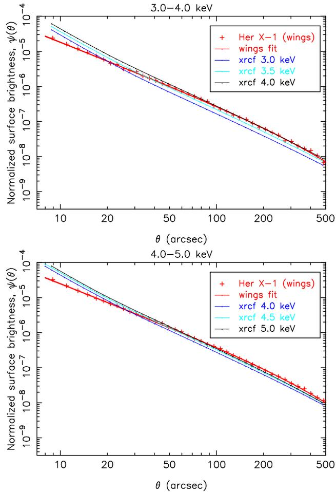
Figure 6: Powerlaw plus exponential cutoff fits to the obsid 3662 (Her X-1 wings) data; the fits were for  $\theta \geq 15''$ . The model based on ground calibration data is also indicated (labeled “xrcf”). Top: 3.0-4.0 keV. Bottom: 4.0-5.0 keV.
