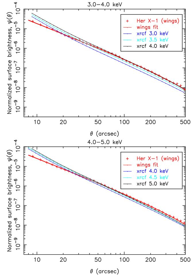
Figure D.2: Powerlaw plus exponential cutoff fits to the obsid 3662 (Her X-1 wings) data; the fits were for  $\theta \geq 15''$ . Mirror vignetting was included in exposure correcting the data (see text). The model based on ground calibration data is also indicated (labeled “xrcf”). Top: 3.0-4.0 keV. Bottom: 4.0-5.0 keV.
