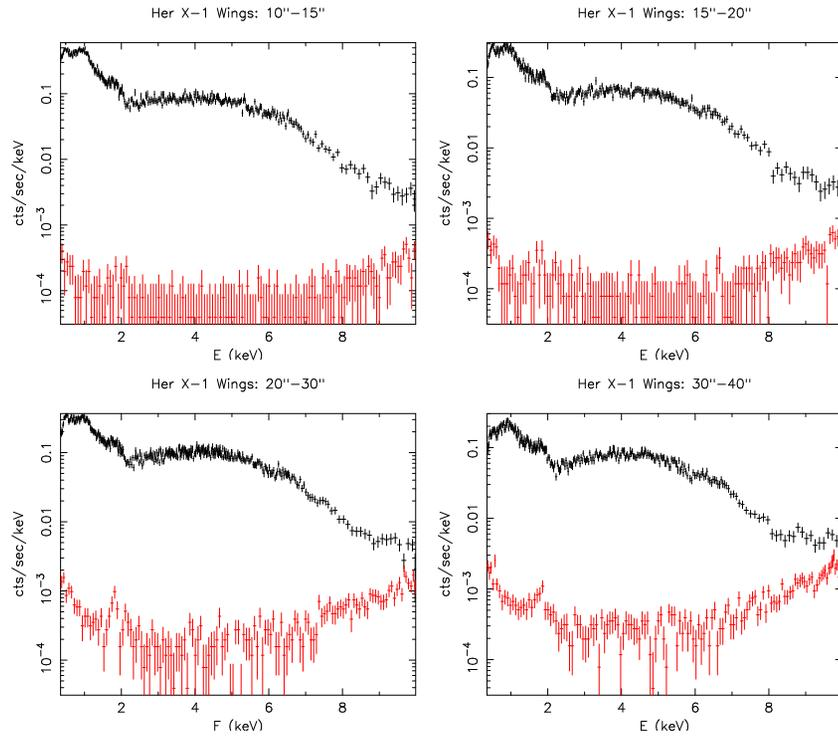
Figure E.2: Spectrum of the Her X-1 diffuse mirror scattering wings (excluding the core ACIS transfer streak). Top Left:  $10'' - 15''$ ; source and blank sky. Top Right:  $15'' - 20''$ ; source and blank sky. Bottom Left:  $20'' - 30''$ ; source and blank sky. Bottom Right:  $30'' - 40''$ ; source and blank sky.
