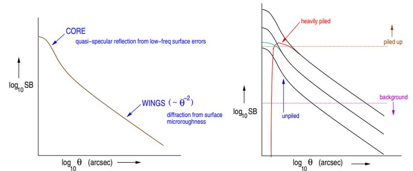
Figure 1: Left: Schematic of the on-axis PSF as a function of angular distance from the core. Right: Schematic of the effects of detector pileup and background. Count rate per pixel above some limit results in pileup. The pileup modifies the event grades (“grade migration”), which for serious enough degradation, results in loss of the event. Detector and sky background limits how low the source count rate per pixel can be detected.
