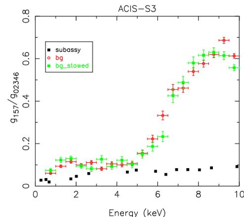
Figure A.1: Ratio of *ASCA* “bad” grades to *ASCA* “good” grades for ACIS-S3 subassembly data and ACIS-S3 on-orbit background data. The *subassy* data are from subassembly calibration test during ground testing. The *bg* and *bg\_stowed* datasets are level 1 background datasets. *bg* is blank sky background, and *bg\_stowed* is background taken when ACIS was out of the focus plane and not exposed to the sky. See text.
