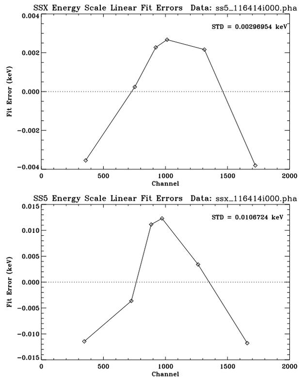
**Figure 5.** SSX and SS5 energy scale linear fit residuals for the flat field test.
