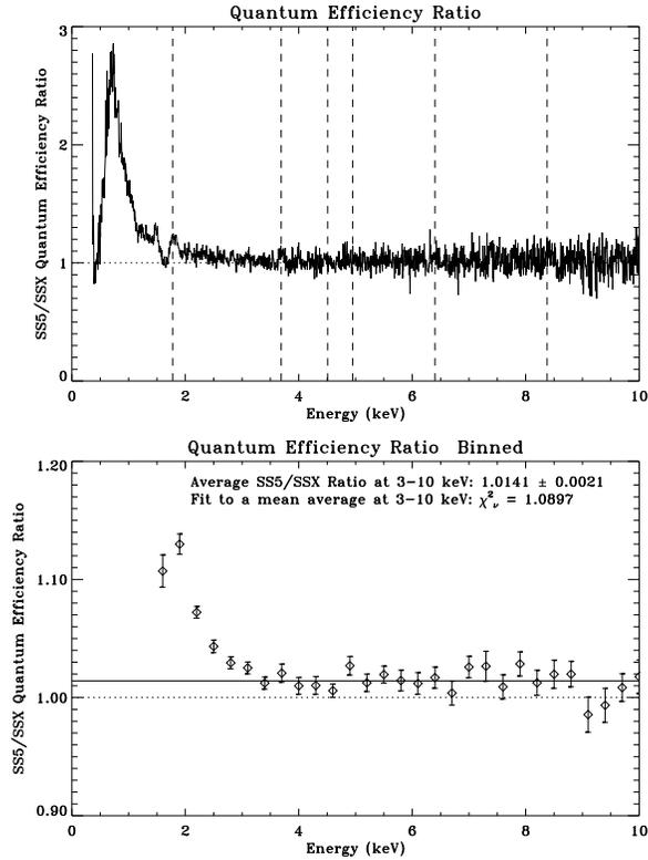
**Figure 9.** SS5/SSX quantum efficiency ratio. In the top panel, the large ratio below 2 keV is mainly due to the different ice build up on the two detectors. The bottom panel shows the ratio curve binned and fitted to a constant ratio. The solid line is the average ratio at 3–10 keV.
