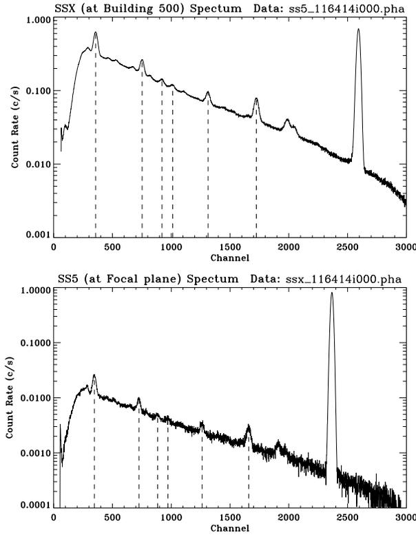
**Figure 3.** C-continuum flat field test SSX and SS5 spectra. Run ID: 116414. 57600 seconds. Dashed vertical lines indicate fitted centers of X-ray characteristic lines to be used for calibrating the SSD energy scale.
