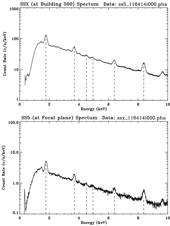
Figure 6. C-continuum flat field test SSX and SS5 spectra as functions of energy, using energy scales from Figure 4.
