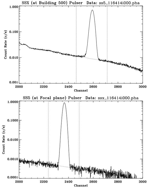
Figure 7. SSX and SS5 pulser spectra. Two vertical dotted lines indicate the pulser region. A dotted line under the peak is the power law fit to the continuum.
