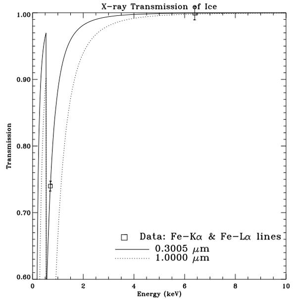
**Figure 11.** X-ray transmission of ice. The solid line is a fit with Fe-L $\alpha$  (0.705 keV) line transmission being 74% of Fe-K $\alpha$  (6.40 keV) line transmission. The result is a 0.3  $\mu\text{m}$  ice layer.
