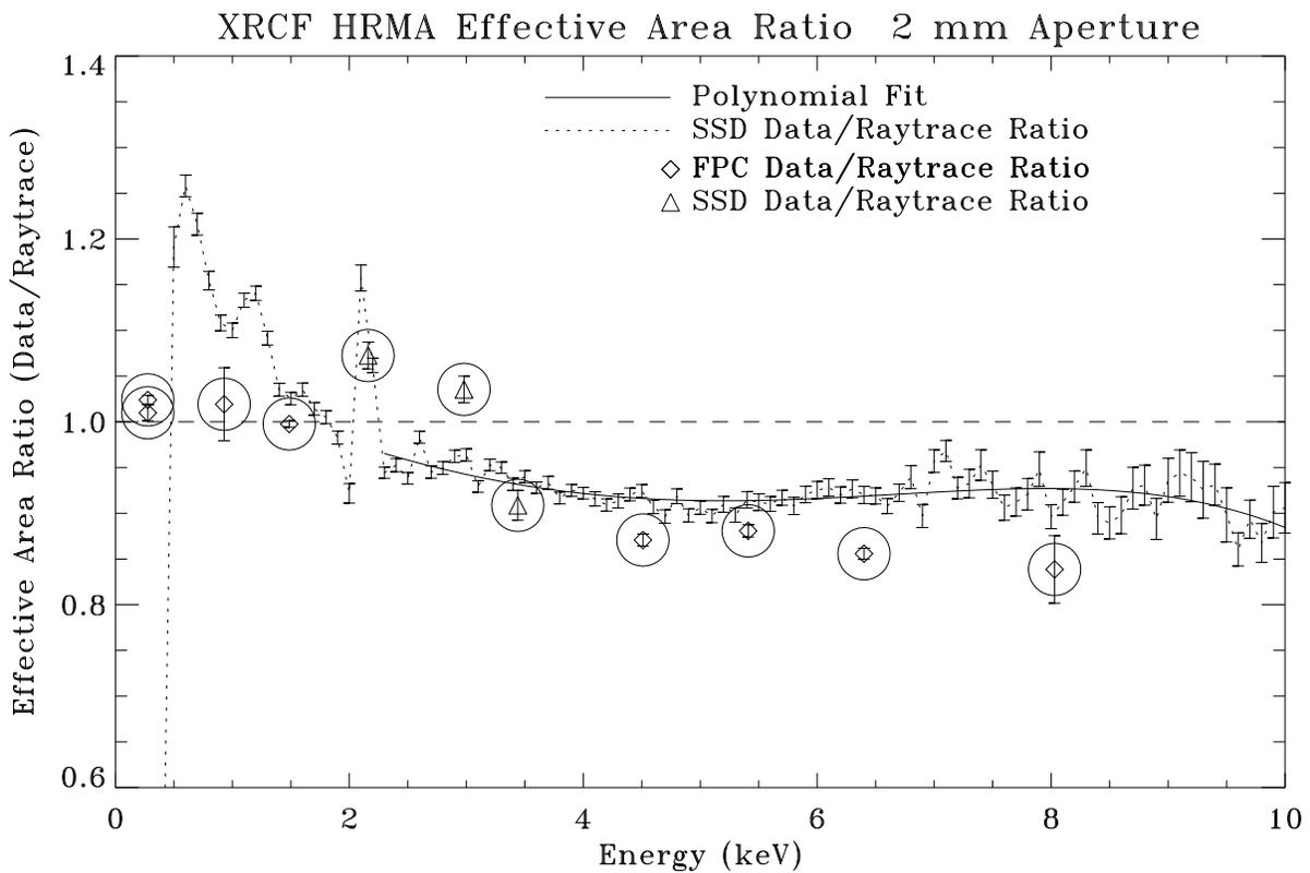
**Figure 17.** Calibration data vs. raytrace prediction. Top panel shows the XRCF HRMA effective area within 2 mm aperture. Bottom panel shows the effective area ratio of data/raytrace.
