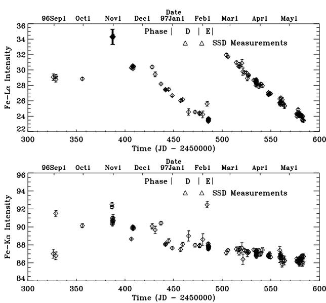
**Figure 10.** SS5 data of Fe-L $\alpha$  and Fe-K $\alpha$  lines from a  $^{244}\text{Cm}$  excited Fe source, used to estimate the ice thickness.
