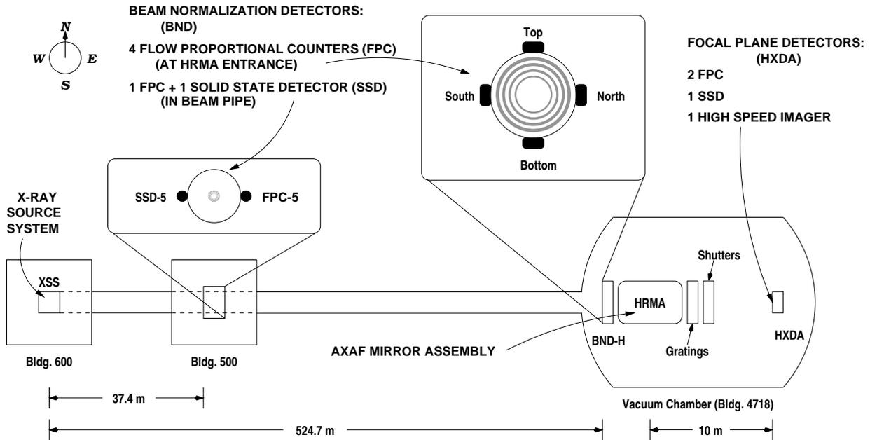
Figure 1. HRMA Calibration configuration at the XRCF.
