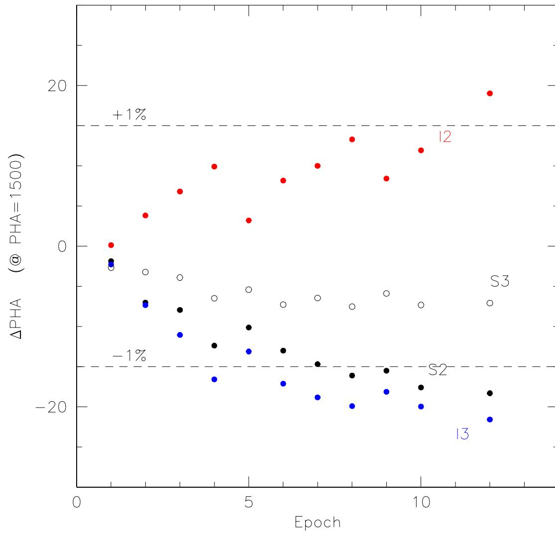
Gain changes ( $\Delta\text{PHA}$  at  $\text{PHA} = 1500$ ) at several representative locations in I2, I3, S2, and S3. Each epoch spans 3 months starting February, 2000. Positive drift in I2 caused by the evolution of the detector gain. — **3-month time resolution is adequate**
