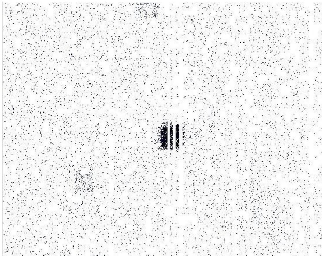
In instrument space, the photons are spread out over 20 arcsec and have bad columns going through them - so be careful of the effective exposure time. If you didn't dither, you could lose the source entirely if it landed on a bad pixel
