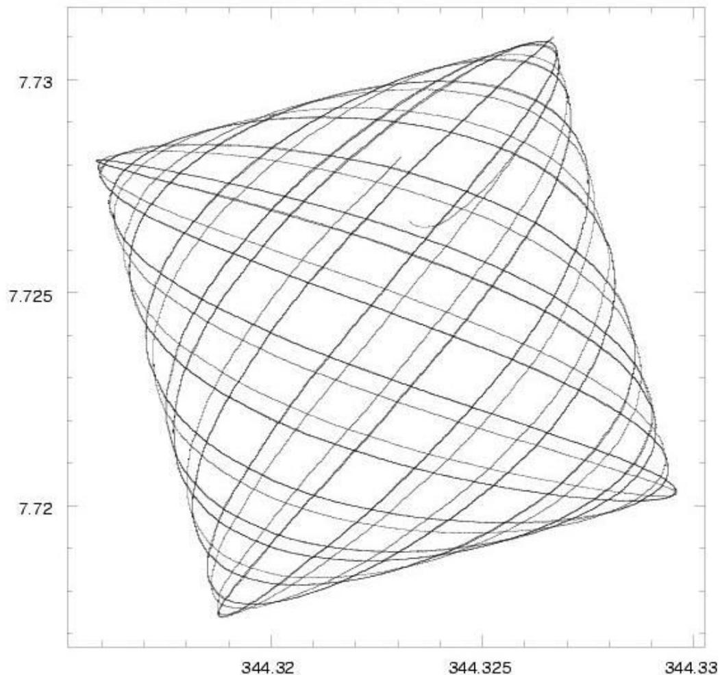
During an observation, Chandra's optical axis describes this 'dither pattern' on the sky, **(Problem 5)**, smearing the image of a point source. The RA, Dec, roll angle of the telescope versus time is called the 'aspect solution'; the asol1.fits file provides this for each observation.
