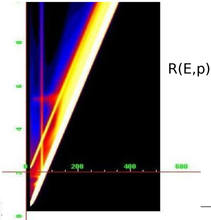
$A(E)$  changes with time (contamination correction) and detector position (quantum efficiency uniformity map); so does the slope of  $R(E,p)$ , the “gain” mapping instrument channel to energy (TGAIN correction, gain map). The width of  $R(E,p)$  changes due to CTI effects. The calibration also changes with CCD operating temperature.
