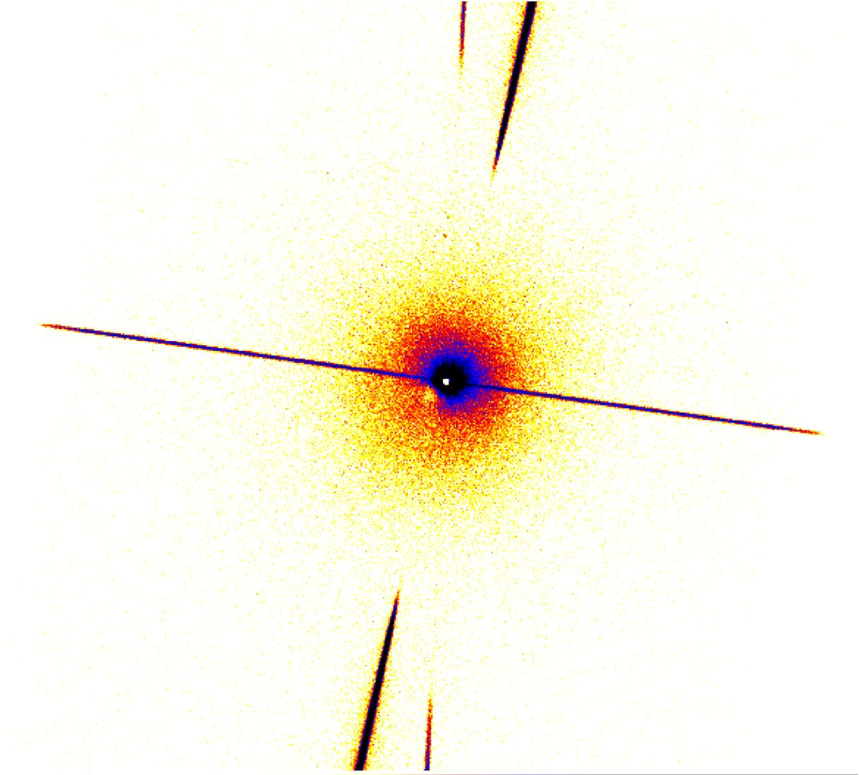
Figure 15. An example of a vertical frame-transfer streak. The streak is vertical in chip, not sky coordinates. In this image, the streak is nearly horizontal. The linear features at the top and bottom are portions of the HETG grating arms.
