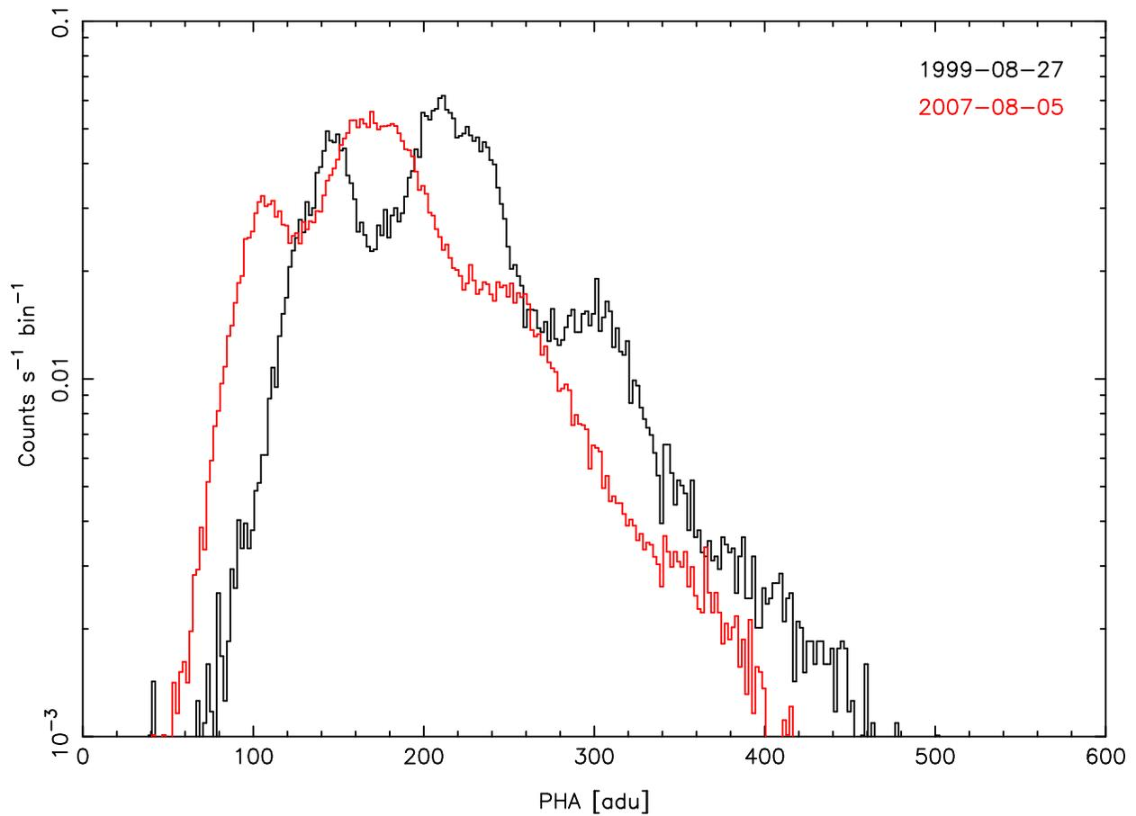
Figure 16. An example of the effects of CTI on the the spectrum of 1E0102.2-7219. Spectra from two separate observations are shown. One is relatively free from the affects of CTI (black histogram). The other has been altered significantly by these effects (red histogram). Note that the red histogram is shifted to lower pulse heights and that it has broader line features.
