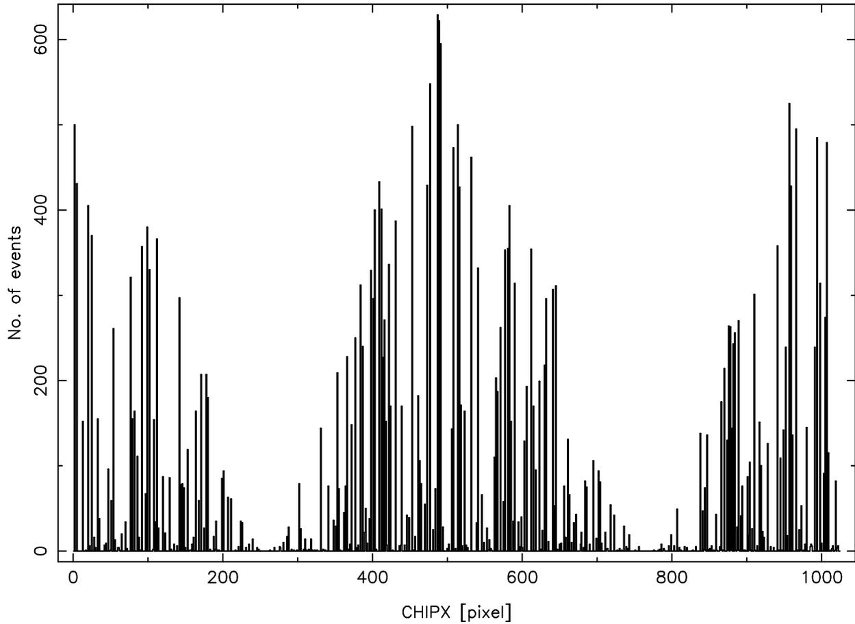
Figure 14. The CHIPX distribution of only the streak events. These events are concentrated closer to the read-out locations at CHIPX = 1, 512, 513, and 1024, than to the opposite ends of the nodes at CHIPX = 256, 257, 768, and 769, respectively.
