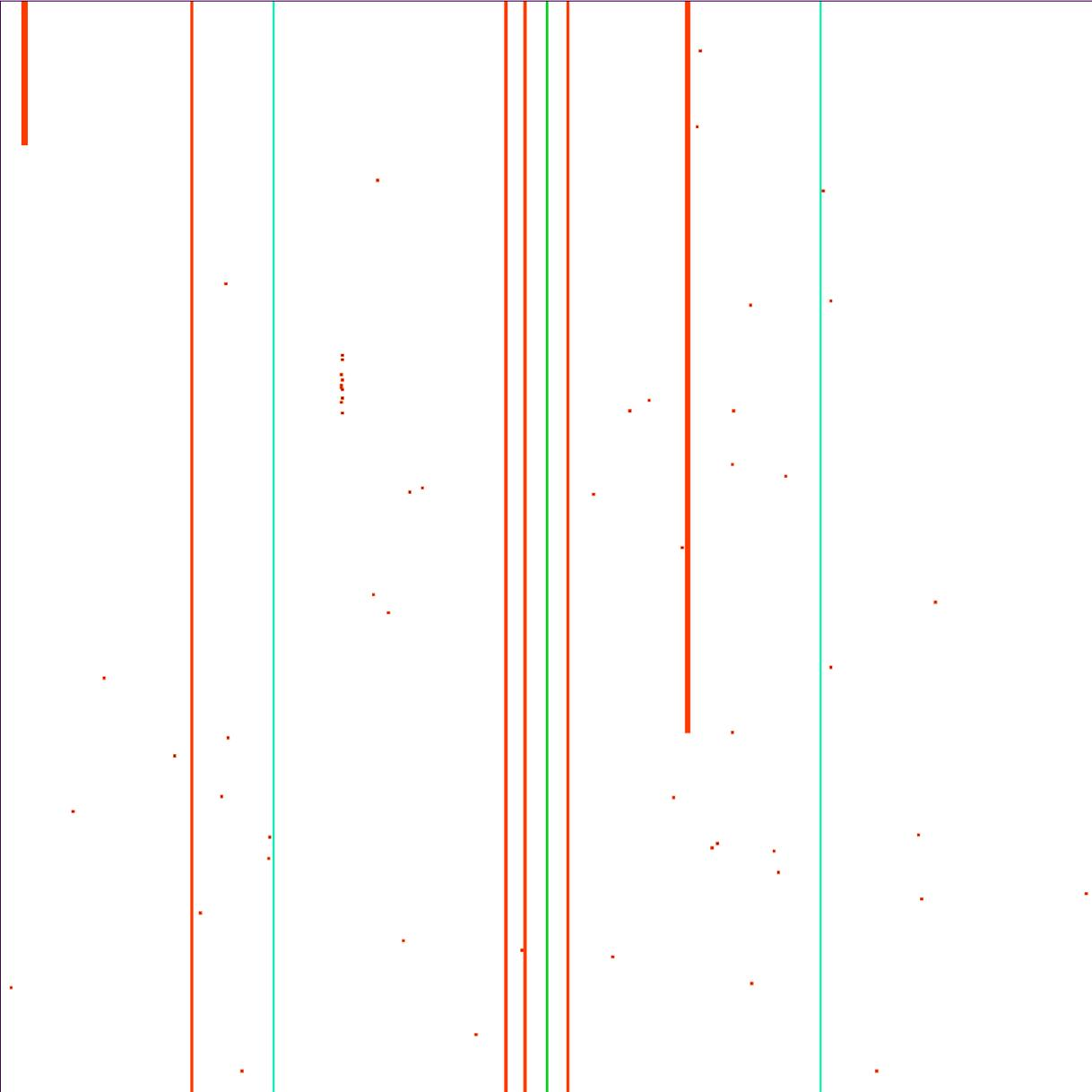
Figure 1. A nominal set of bad pixels for the CCD ACIS-I3. Different types of bad pixels are color coded. However, not every type of bad pixel has a unique color.
