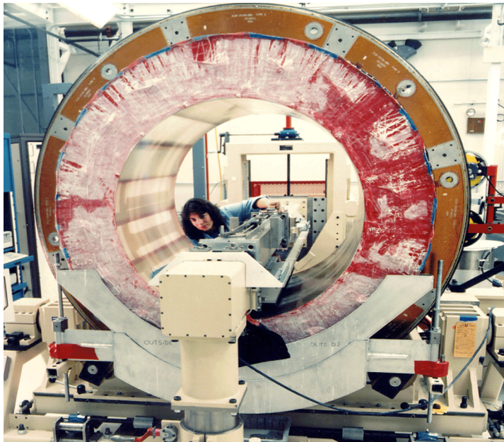
Polishing a CXO Mirror Shell
