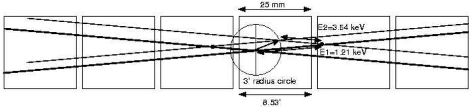
Figure 8.25: An idealized sketch of a 'collision' between two sources separated by 3 arcmin. At the 'collision' point, third-order photons from the on-axis source will have an energy  $3 \times 1.21 = 3.63$  keV and ACIS can not distinguish these from the second source's first order photons, at 3.64 keV.
