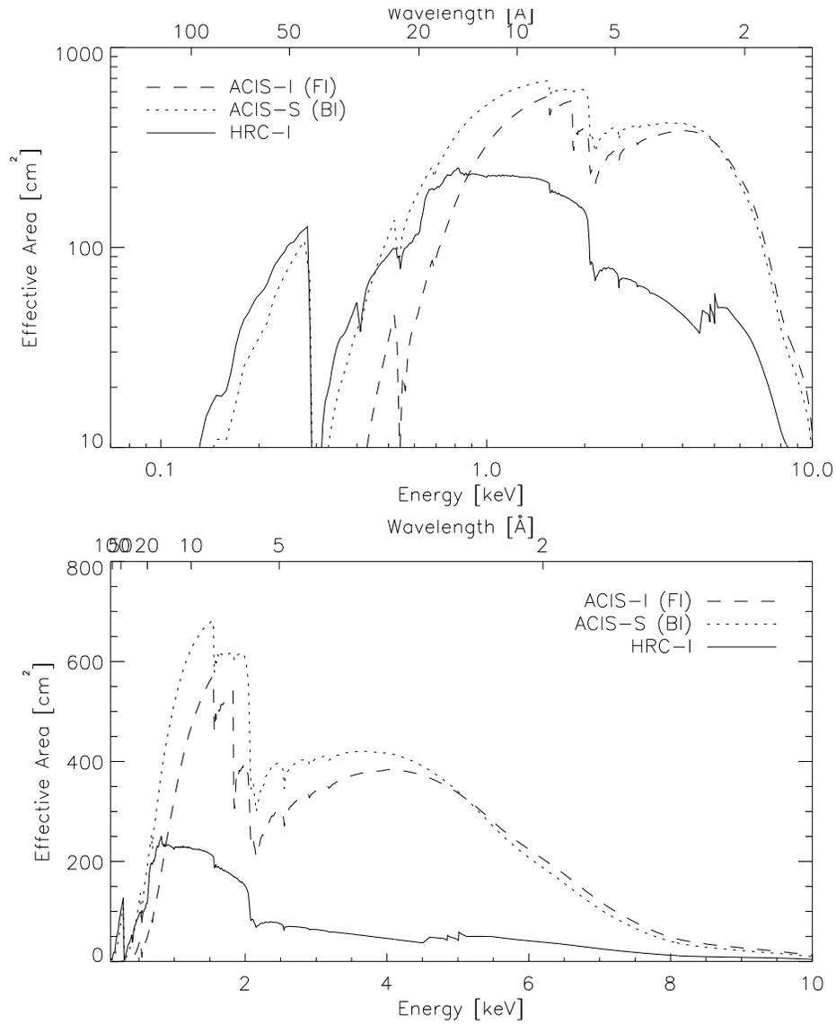
Figure 1.3: Comparison of the on-axis effective areas for observing a point source (integrated over the *PSF*) of the HRMA/HRC-I, the HRMA/ACIS(FI), and the HRMA/ACIS(BI) combinations. The ACIS curves show the predicted values for the middle of Cycle 12 (2010-05-15).
