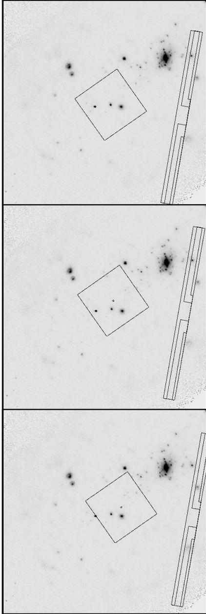
Figure 3.2: Example of offset pointing with HRC. North is up and East is to the left. Roll is measured positive, West of North. The roll angle shown is  $10^\circ$ . Left Panel: The target, the middle source in a group of three aligned N-S, is at the nominal HRC-I aimpoint. Center Panel: The target is offset with  $(Y, Z)$  offset of  $(-5, 0)$  arcmin. Right Panel: The offset is  $(-5, -5)$ . Note the small dot at the location of the HRC-I aimpoint.
