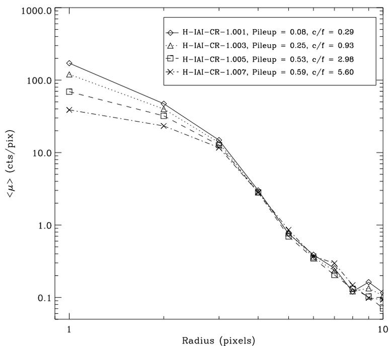
Figure 6.17: The effects of pileup on the radial distribution of the *PSF* are illustrated. These data were taken during ground calibration at the XRCF. The specific “OBSIDs”, the counting rate per CCD frame (“c/f”), and the “pileup fraction” as defined in Section 6.15.2 are given in the inset.
