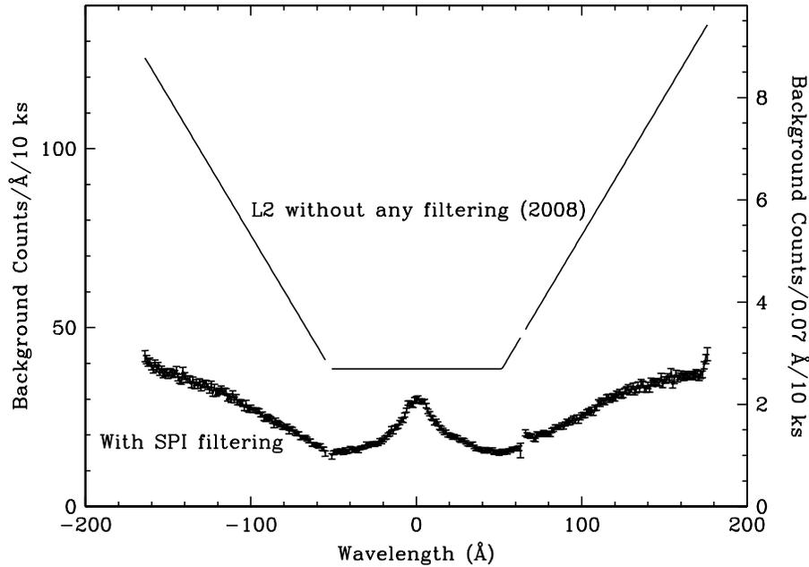
Figure 9.21: The LETG+HRC-S background rate with and without the new SPI filter. Data are shown using the standard ‘bowtie’ spectral extraction region (see Figure 9.14). X-ray losses from the observed spectrum as a result of the filtering for 1st order are  $\sim 1.25\%$ ; losses will be slightly higher for higher orders. See [http://cxc.harvard.edu/cal/Letg/Hrc\\_bg](http://cxc.harvard.edu/cal/Letg/Hrc_bg) for more information.
