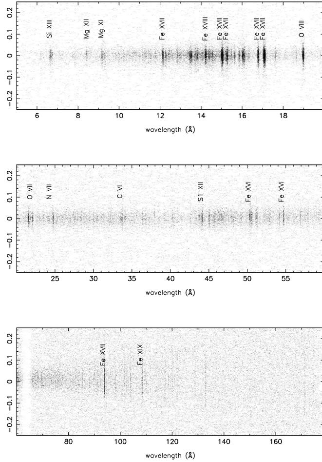
Figure 9.24: HRC-S detector image of a Capella observation, showing positive order dispersion. Both axes are in  $\text{\AA}$  with  $1.148 \text{ \AA}/\text{mm}$ . The increasing cross-dispersion extent of lines at longer wavelengths is due to astigmatism in the HRMA/LETG system. The positive-order HRC-S plate gap is at  $\sim 63 \text{ \AA}$ .
