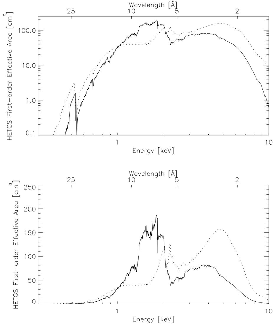
Figure 8.11: The modeled total first-order (solid curve) and zeroth-order (dotted curve) effective area, integrated over the PSF, of the **HRMA-HETG-ACIS-S** combination, as a function of energy. The first-order data are the same as those plotted in Figures 8.7 and 8.9. The plotted first-order values are the sums of the area at a particular energy from both orders (+/-) of both MEG and HEG spectra. Both a log-log and a log-linear version are shown.
