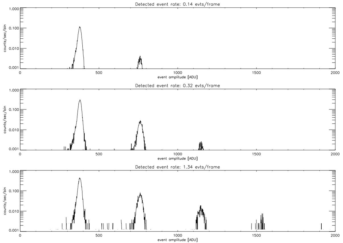
Figure 6.18: The effects of pileup at 1.49 keV ( $\text{Al K}\alpha$ ) as a function of source intensity. Data were taken during HRMA-ACIS system level calibration at the XRCF. Single-photon events are concentrated near the pulse height corresponding to the  $\text{Al K}\alpha$  line ( $\sim 380$  ADU), and events with 2 or more photons appear at integral multiples of the line energy.
