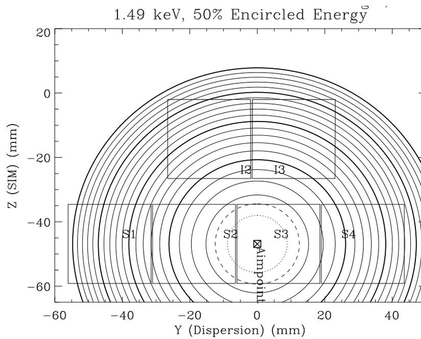
Figure 6.12: Approximate contours of constant 50% encircled energy at 1.49 keV when the ACIS-S default aimpoint is selected. The dotted line is 1 arcsec, the dashed line is 1.5 arcsec. The remainder are at 1 arcsec intervals. The thicker solid lines highlight the 5, 10, 15 and 20 arcsec contours.
