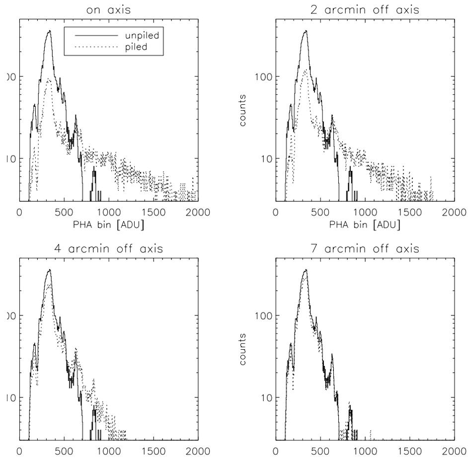
Figure 6.21: MARX simulations of the effect of pileup on the shape of the spectrum. The true (solid line) and the detected (dotted line) spectra are shown for four different viewing angles. The corresponding “pileup fractions” - see Section 6.15.2 - are 46%, 40%, 15%, and 2% as the image is moved progressively further off-axis.
