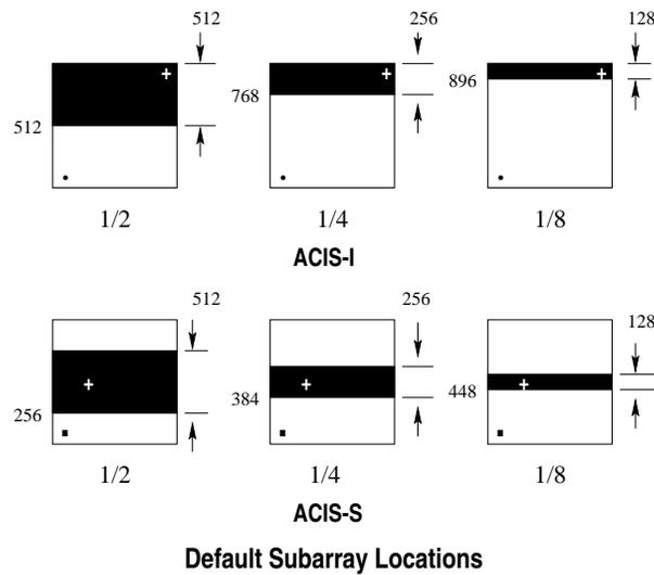
Figure 6.15: Examples of various subarrays. The heavy dot in the lower left indicates the origin
