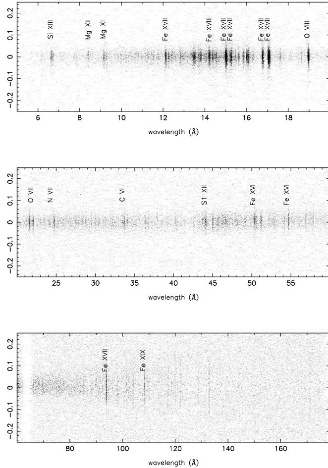
Figure 9.25: HRC-S detector image of a Capella observation, showing positive order dispersion. Both axes are in  $\text{\AA}$  with  $1.148 \text{ \AA}/\text{mm}$ . The increasing cross-dispersion extent of lines at longer wavelengths is due to astigmatism in the HRMA/LETG system. The positive-order HRC-S plate gap is at  $\sim 63 \text{ \AA}$ .
