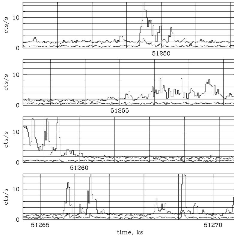
Figure 6.27: An example of the ACIS background counting rate versus time - BI chip (S3; top curve) and an FI chip (I2; bottom curve). These are for the standard grades and the band from 0.3 - 10 keV.
