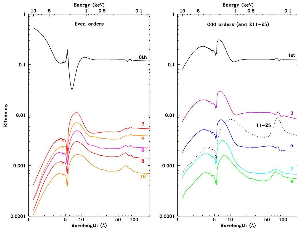
Figure 9.13: LETGS grating efficiency. Combined positive and negative order efficiency is plotted versus wavelength and energy. For clarity, even and odd orders are plotted separately; the sum of orders 11–25 is also shown. Plotted values include all support structure diffraction. Net efficiency when using a spectral extraction region (see Figures 9.14 and 9.15) is 10–15% lower. Features near 6 and 80 Å are due to the partial transparency of the gold grating material at these wavelengths.
