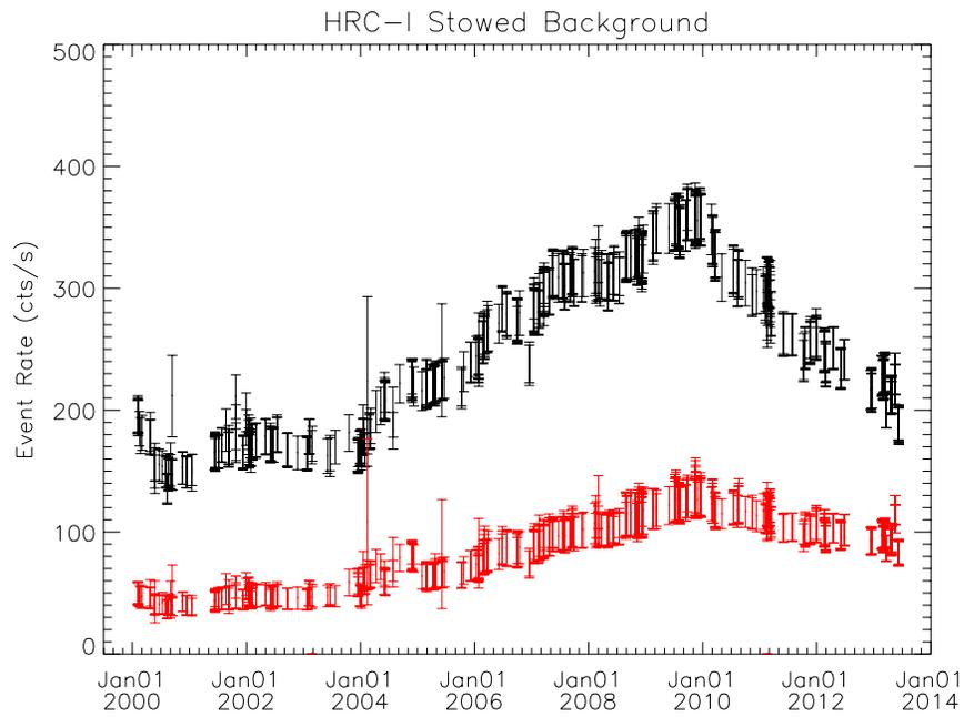
Figure 7.19: The change in HRC-I stowed background rate with time. The total rate (black points and error bars, upper set) and the valid rate (red points and error bars, lower set) are shown. The HRC-S data are similar.
