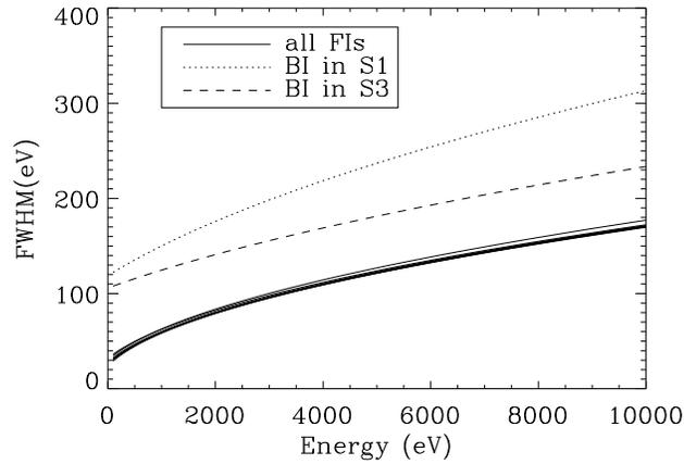
Figure 6.9: The ACIS pre-launch energy resolution as a function of energy.
