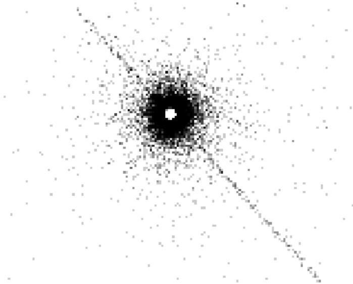
Figure 6.16: Trailed image of a strong X-ray source. The core of the image is faint due to pileup. Most events here are rejected because of bad grades. The readout direction is parallel to the trail.
