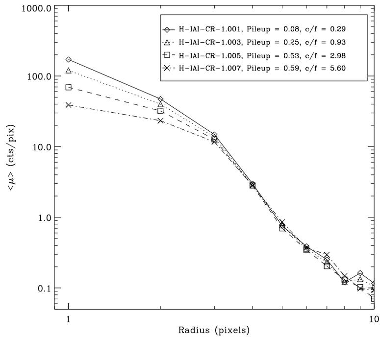
Figure 6.19: The effects of pileup on the radial distribution of the PSF are illustrated. These data were taken during ground calibration at the XRCF. The specific “OBSIDs”, the counting rate per CCD frame (“c/f”), and the “pileup fraction” as defined in Section 6.15.2 are given in the inset.
