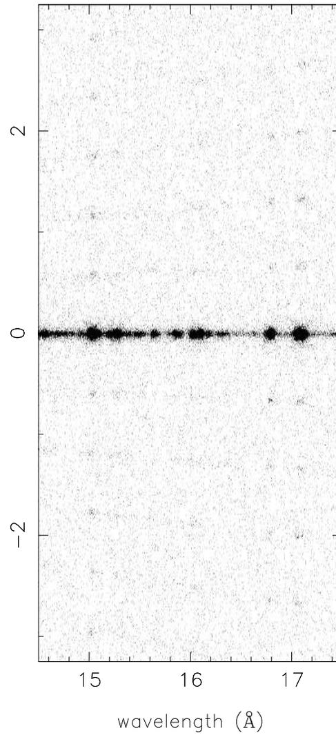
Figure 9.24: Detail of Figure 9.23, showing the LETG/HRC-S image of bright lines in Capella. Both axes are in  $\text{\AA}$  with  $1.148 \text{ \AA/mm}$ . The Fe XVII lines at  $\sim 15$  and  $17 \text{ \AA}$  are the brightest in the LETG Capella spectrum. Faint features above and below the primary spectrum are due to fine support structure diffraction.
