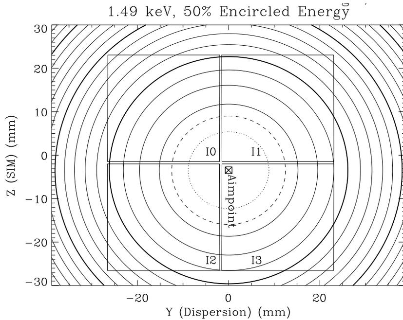
Figure 6.11: Approximate contours of constant 50% encircled energy at 1.49 keV when the ACIS-I default aimpoint is selected. The dotted line is 1 arcsec, the dashed line is 1.5 arcsec. The remainder are at 1 arcsec intervals. The thicker solid lines highlight the 5, 10, and 15 arcsec contours.
