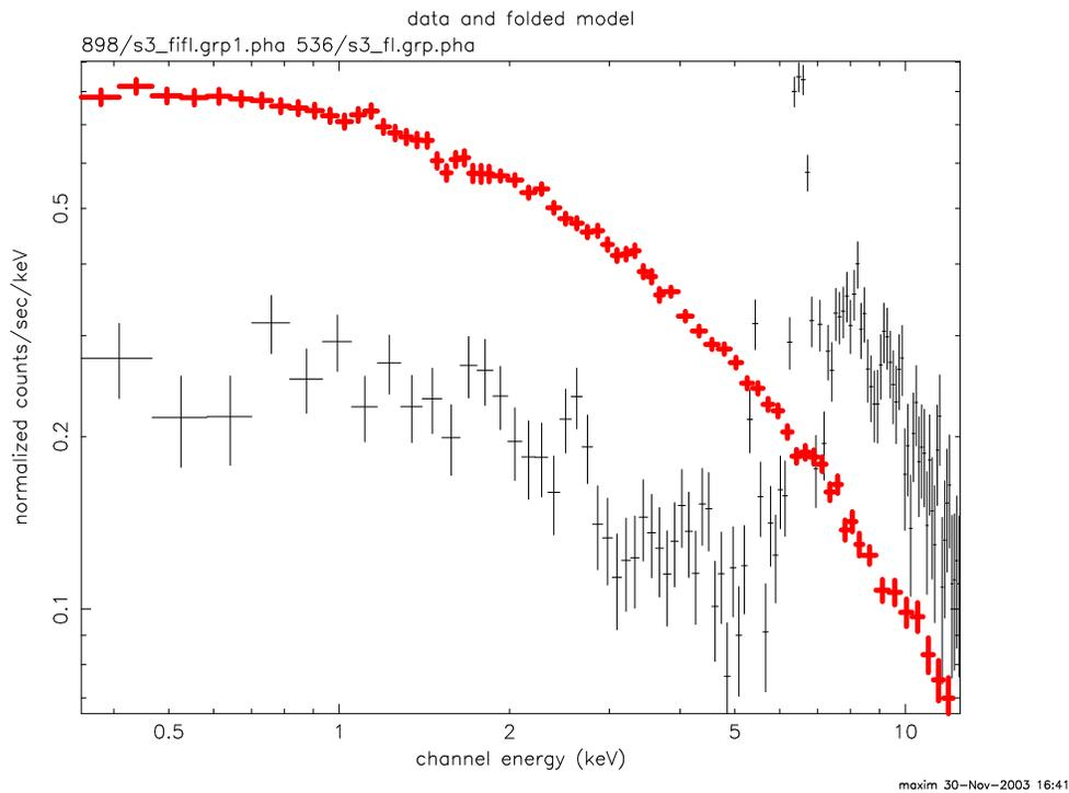
Figure 6.29: Spectra of different background flares in chip S3. Thick crosses show a common flare species that affects only the BI chips. Thin crosses show one of the several less common flare species that affect both the BI and FI chips. Note how both these spectra are different from the quiescent spectrum (see Figure 6.23).
