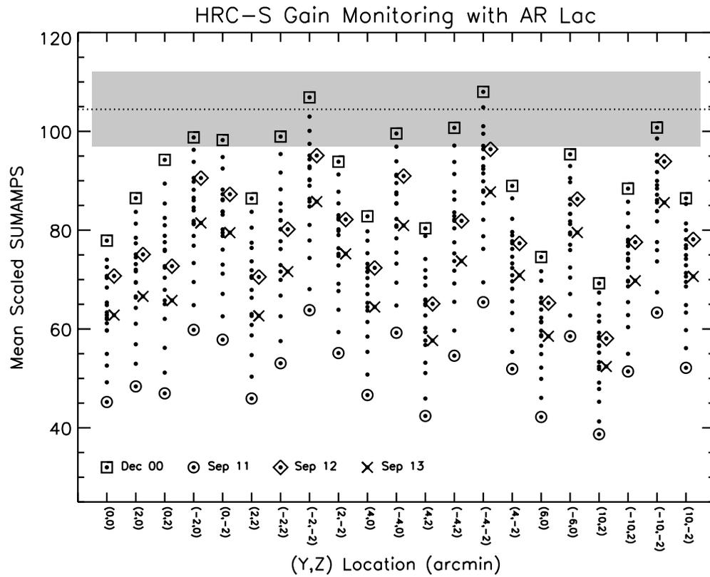
Figure 7.14: Monitoring the gain and gain correction across the HRC-S detector. The mean scaled SUMAMPS at each epoch (solid points) declined with time at all pointings from the beginning of the mission (square symbols) till before the voltage change (circle symbols). After the voltage was increased in March 2012, the mean SUMAMPS increased (diamond symbols) to nearly the same level as at the beginning of the mission.
