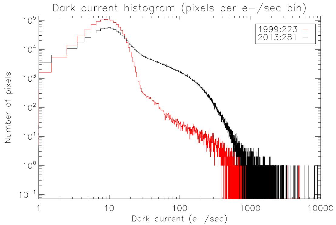
Figure 5.6: Differential histogram of dark current distribution for the ACA CCD in 1999-Aug and 2013-Oct
