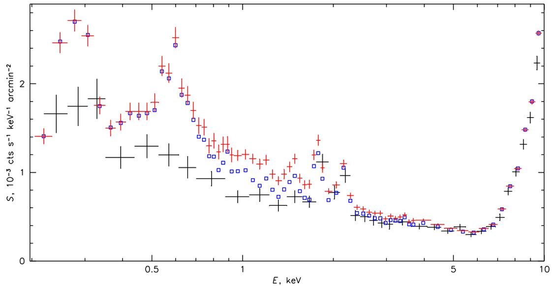
Figure 6.25: ACIS -S3 spectrum of the non-X-ray background (large crosses) overlaid on the quiescent blank sky spectrum. Small crosses show the total sky spectrum, while squares show the diffuse component left after the exclusion of all point sources detectable in this 90 ks exposure. Standard grade filtering and VF filtering are applied. The background and blank-sky spectra are normalized to the same flux in the 10-12 keV band.
