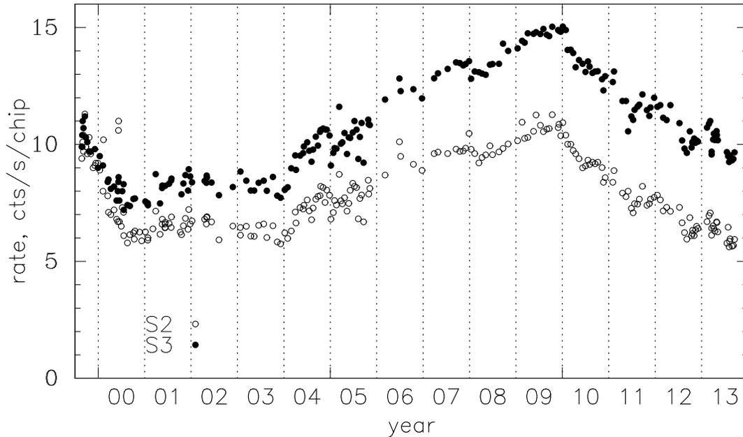
Figure 6.26: Total telemetered background rates (including all grades and the upper event cutoff at 15 keV) for chips S2 (FI) and S3 (BI) as a function of time. Vertical dashed lines are year boundaries.
