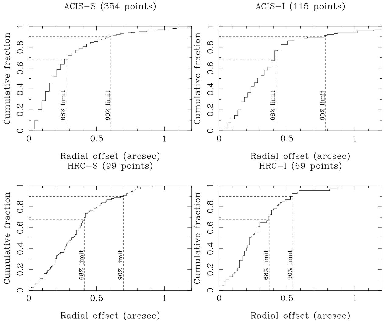
Figure 5.4: Cumulative histogram of celestial accuracy for *Chandra* X-ray source locations for each SI. Radial offset is the distance in arcsec between the optical coordinate, typically from the Tycho-2 catalog, and the *Chandra* position.
