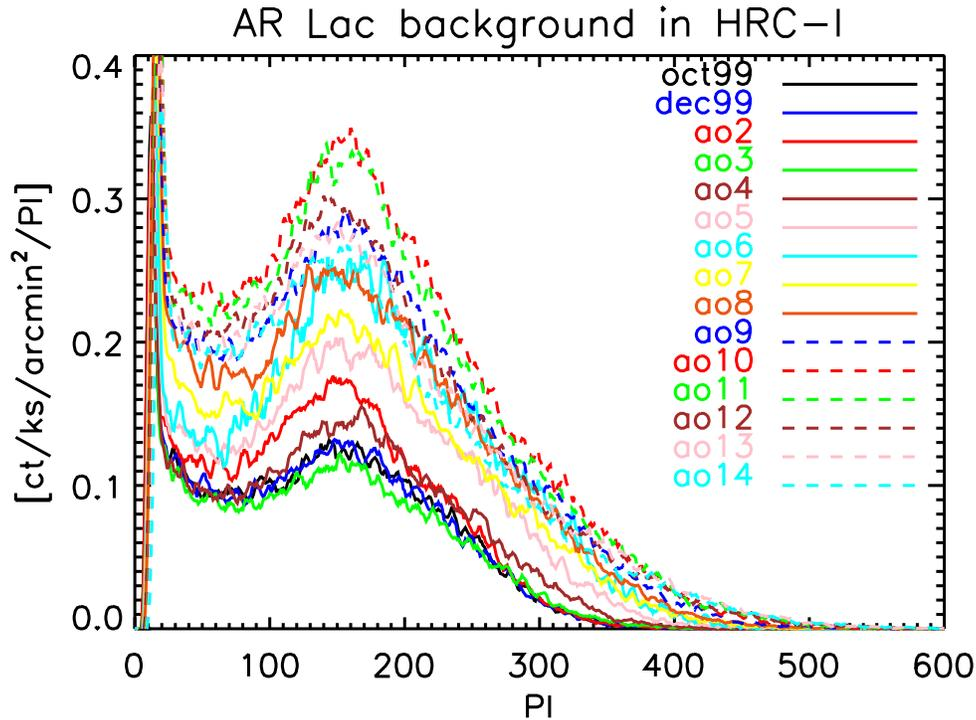
Figure 7.18: Average background spectra in the inner  $10'$  region of the detector, obtained from yearly observations towards AR Lac are shown. Times of high background flaring have been excluded. The magnitude and shape of the spectra vary considerably with time, but may be interpolated between epochs to estimate the background for any given observation.
