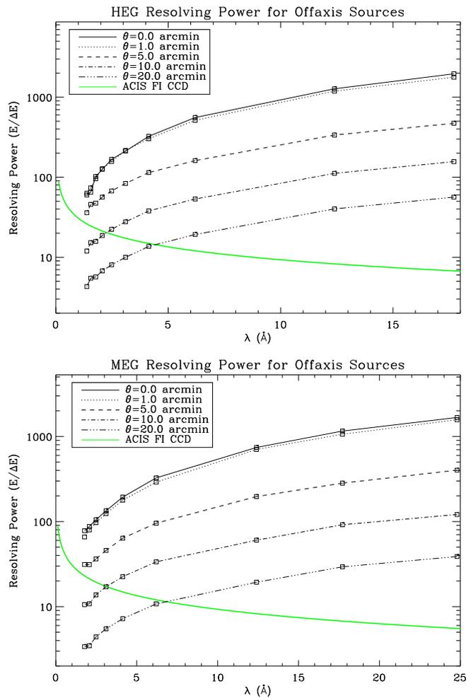
Figure 8.24: The effects of off-axis pointing on the HETG grating spectral resolution. Using *MARX*, we have simulated an observation of a point source at increasing off-axis positions. The effect on the resolving power ( $E/\Delta E$ ) is shown as a function of photon energy for off-axis angles of  $0'$ ,  $1'$ ,  $5'$ ,  $10'$ , and  $20'$ . The spectral resolution of an ACIS Front Illuminated (FI) CCD at a point near the framestore region is shown for comparison.
