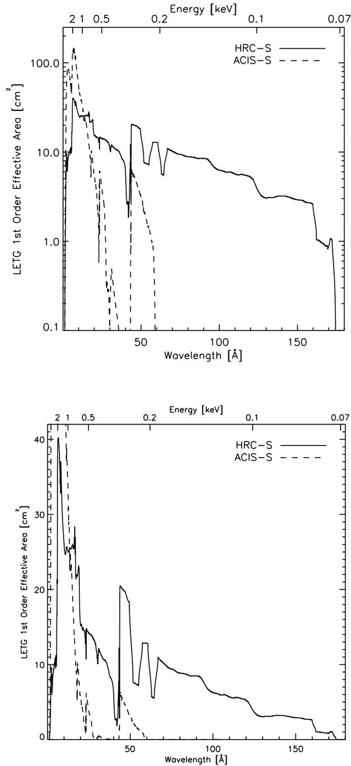
Figure 9.17: LETGS 1st-order effective area for an on-axis point source, with HRC-S and ACIS-S detector configurations with log (top) and linear (bottom) scaling. Positive and negative orders are summed. LETG+ACIS-S areas were computed using an effective area model that included the effects of contamination build-up extrapolated to the level expected in mid-2015. Note that the vertical scale of the linear plot has been truncated.
