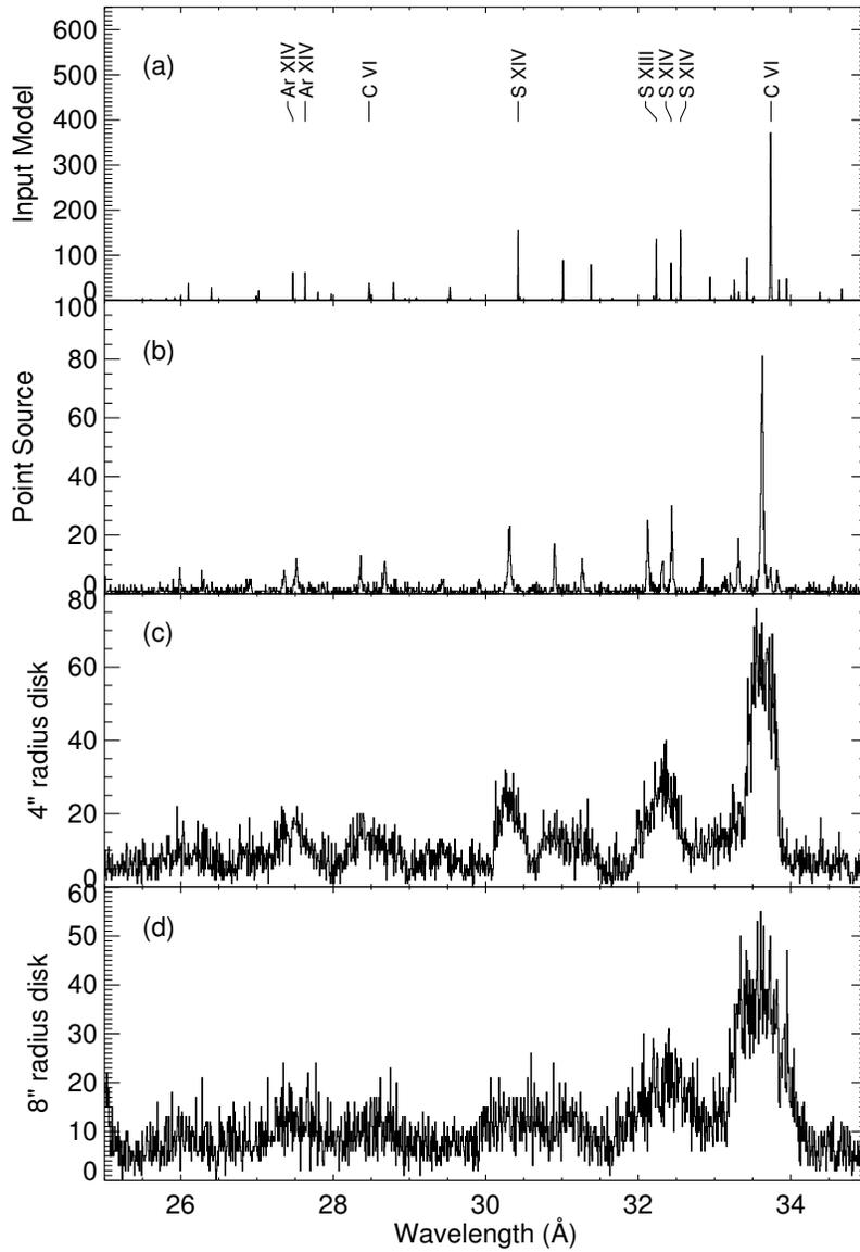
Figure 9.30: *MARX* simulation of spectra showing the effect of source extent. The panels show (a) computed input spectrum, (b) a *MARX* output of LETG spectrum of a point source, (c) the same as (b) except that the source is a disc of uniform brightness with radius of  $4''$ , and (d) the same but with radius of  $8''$ . See Figure 9.11 and Section 9.3.3 for a discussion of extended sources.
