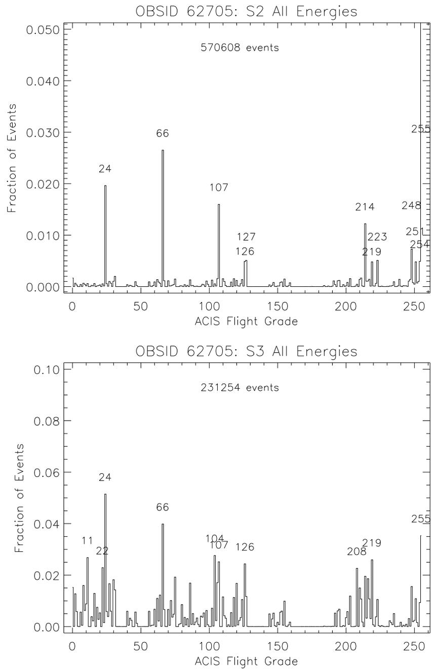
Figure 6.24: Fraction of ACIS background events as a function of grade from early in-flight data for an FI chip (S2) (top) and a BI chip (S3) (bottom).
