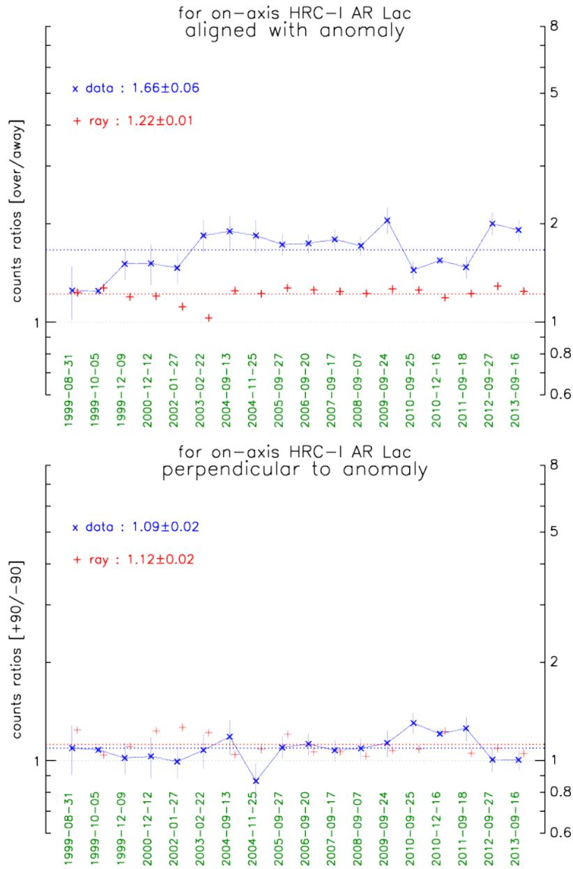
Figure 4.19: As Figure 4.18, for on-axis HRC-I observations of AR Lac. Notice that the magnitude of the anomaly was low early in the mission and appears to be fully formed by Feb 2003. There are also indications that the asymmetry was reduced between late-2010 till late-2011. The ray trace PSF model for the HRC includes smoothing due to detector blur.
