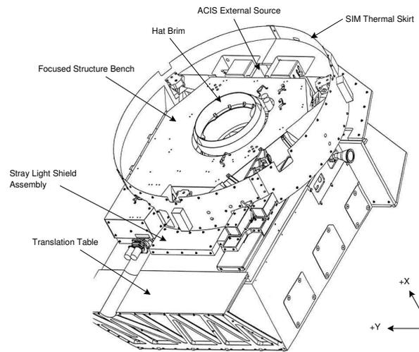
Figure 2.1: A schematic of the Science Instrument Module.
