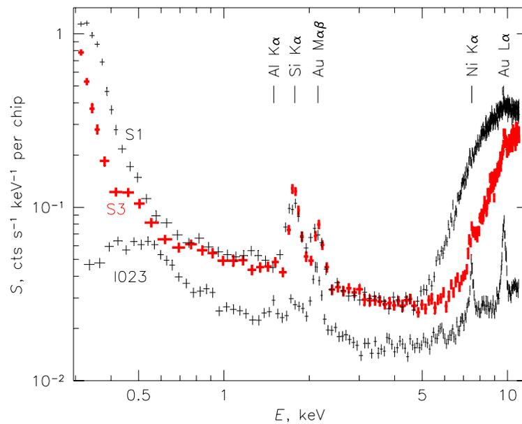
Figure 6.23: Energy spectra of the charged particle ACIS background with ACIS in the stowed position (a 50 ks exposure taken in September 2002; standard grade filtering, no VF filtering). Line features are due to fluorescence of material in the telescope and focal plane.
