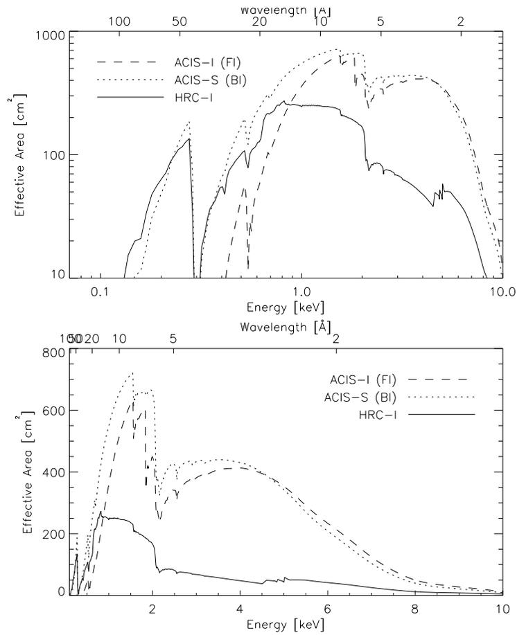
Figure 1.3: Comparison of the on-axis effective areas for observing a point source (integrated over the *PSF*) of the HRMAHRC-I, the HRMA/ACIS(FI), and the HRMA/ACIS(BI) combinations. The ACIS curves show the predicted values for the middle of Cycle 9 (2008-05-15).
