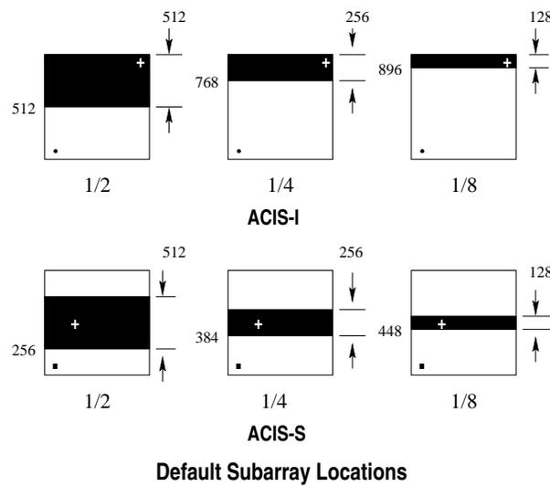
Figure 6.13: Examples of various subarrays. The heavy dot in the lower left indicates the origin
