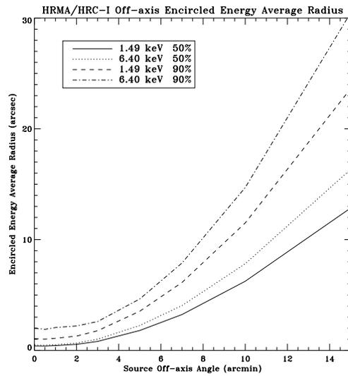
Figure 7.6: Encircled energy as a function of source off-axis angle for 50% and 90% encircled energy for 1.49 and 6.40 keV for the combined **HRMA**/HRC-I. A conservative contribution from the aspect solution is included ( $\text{FWHM} = 20 \mu\text{m}$  ( $0.41''$ )). A plot for the combined **HRMA**/HRC-S would be almost identical since the PSFs of the two instruments are virtually identical and independent of off-axis angle.
