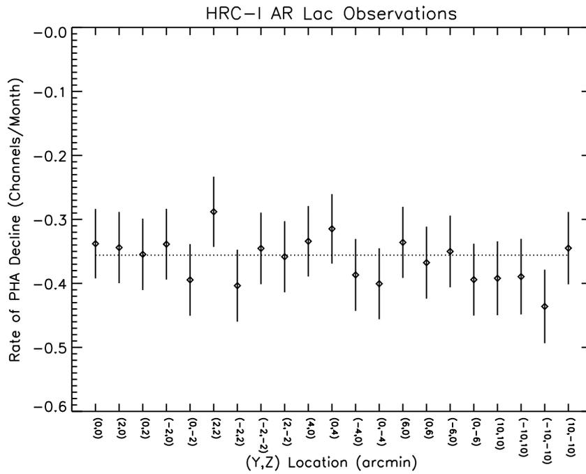
Figure 7.14: The rate of change of the median PHA derived for AR Lac observations carried out at numerous locations across the HRC-I detector, based on observations from Cycles 2-7. The PHA values are corrected for spatial variations separately for each set of observations. The dotted horizontal line represents the mean value of the gain drop.
