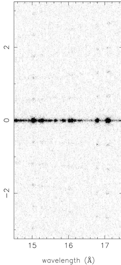
Figure 9.23: Detail of Figure 9.22, showing the LETG/HRC-S image of bright lines in Capella. Both axes are in  $\text{\AA}$  with  $1.148 \text{ \AA}/\text{mm}$ . The Fe XVII lines at  $\sim 15$  and  $17 \text{ \AA}$  are the brightest in the LETG Capella spectrum. Faint features above and below the primary spectrum are due to fine support structure diffraction.
