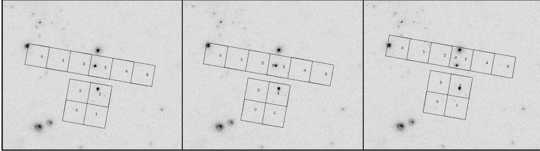
Figure 3.1: Examples of offset pointing with ACIS. North is up and East is to the left. Roll is measured positive, West of North. The roll angle shown is  $10^\circ$ . Left Panel: The target, a bright x-ray source, is centered at the nominal ACIS-S aimpoint. Middle Panel: The target is offset with (Y,Z) offset of  $(-1,0)$  arcmin. In the Right Panel the offset is  $(-1,-3)$ . Note the small circle at the location of the ACIS-S aimpoint.
