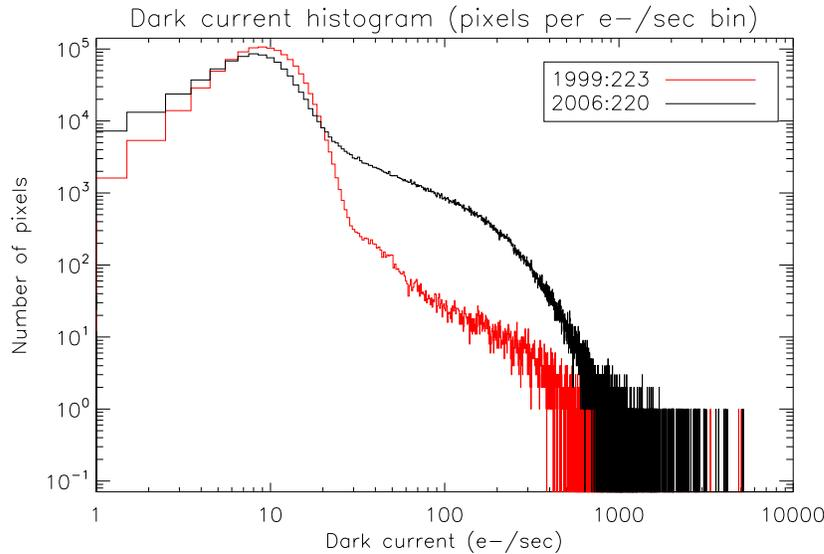
Figure 5.6: Differential histogram of dark current distribution for the ACA CCD in 1999-Aug (gray) and 2006-Aug (black)
