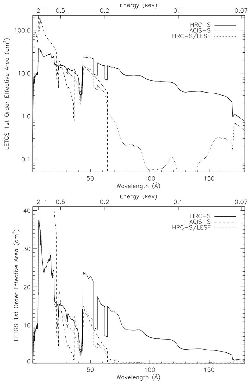
Figure 9.17: LETGS 1st-order effective area for an on-axis point source, with HRC-S, HRC-S LESF and ACIS-S detector configurations with log and linear scaling. Positive and negative orders are summed. LETG+ACIS-S areas were computed using an effective area model that included the effects of contamination build-up extrapolated to the level expected in mid-May 2008. Note that the vertical scale of the linear plot has been truncated.
