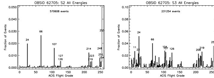
Figure 6.22: Fraction of ACIS background events as a function of grade from early in-flight data for an FI chip (S2) (left) and a BI chip (S3) (right).
