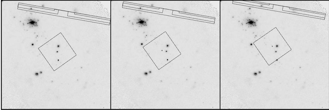
Figure 3.2: Example of offset pointing with HRC. North is up and East is to the left. Roll is measured positive, West of North. The roll angle shown is  $10^\circ$ . Left Panel: The target, the middle source in a group of three aligned N-S, is at the nominal HRC-I aimpoint. Center Panel: The target is offset with (Y,Z) offset of (-5,0) arcmin. Right Panel: The offset is (-5,-5). Note the small dot at the location of the HRC-I aimpoint.
