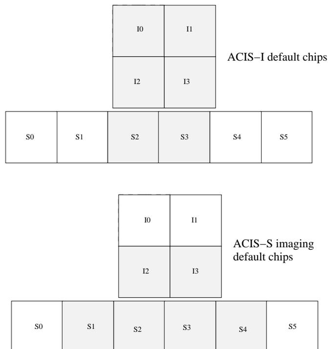
Figure 6.2: A schematic drawing of the ACIS focal plane, not to scale. The ACIS-I array consists of chips I0-I3. Chips S2 and S3 are often turned in addition to I0-I3 when ACIS-I is used in imaging mode as indicated in the top figure. ACIS-S consists of chips S0-S5. When operated in imaging mode chips S1-S4 plus I2 and I3 are often turned on (bottom figure). When operated in spectroscopy mode S0-S5 are usually turned on. See 6.19.1 for more details on chip choices.
