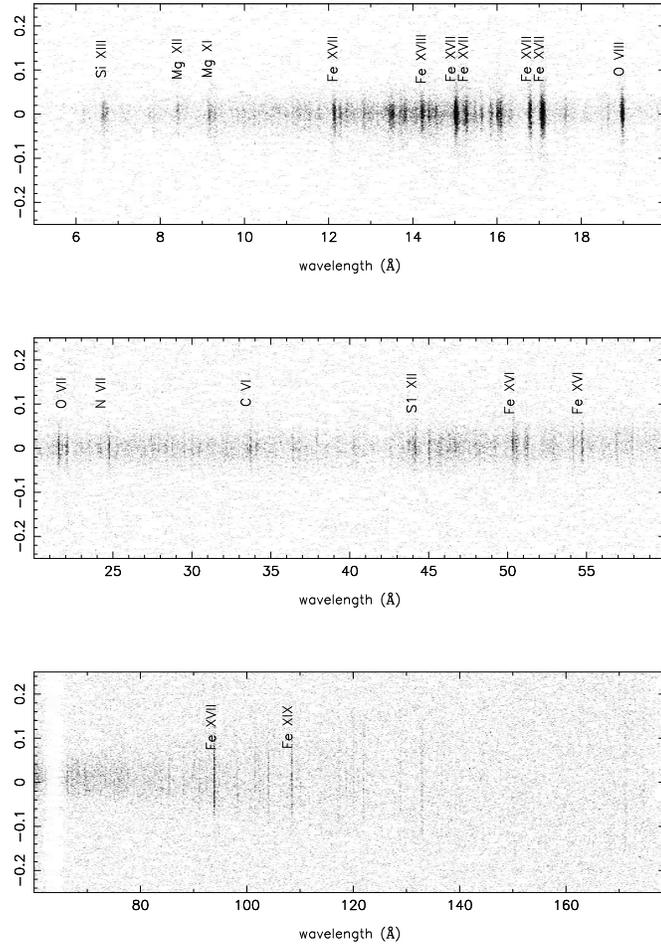
Figure 9.24: HRC-S detector image of a Capella observation, showing positive order dispersion. Both axes are in  $\text{\AA}$  with  $1.148 \text{ \AA/mm}$ . The increasing cross-dispersion extent of lines at longer wavelengths is due to astigmatism in the HRMA/LETG system. The positive-order HRC-S plate gap is at  $\sim 63 \text{ \AA}$ .
