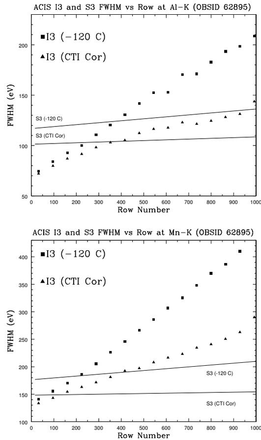
Figure 6.9: An example of the application of the *CXC* CTI-corrector in two energy bands. The upper plot shows data for the Al-K line, and the lower for Mn-K. The square data points are the FWHM of lines averaged over 32-row bins. The triangle data points are the FWHM of CTI-corrected lines. The upper line shows the uncorrected performance of the S3 chip, while the lower line shows the CTI-corrected performance of the S3 chip. These data are from March 2000.
