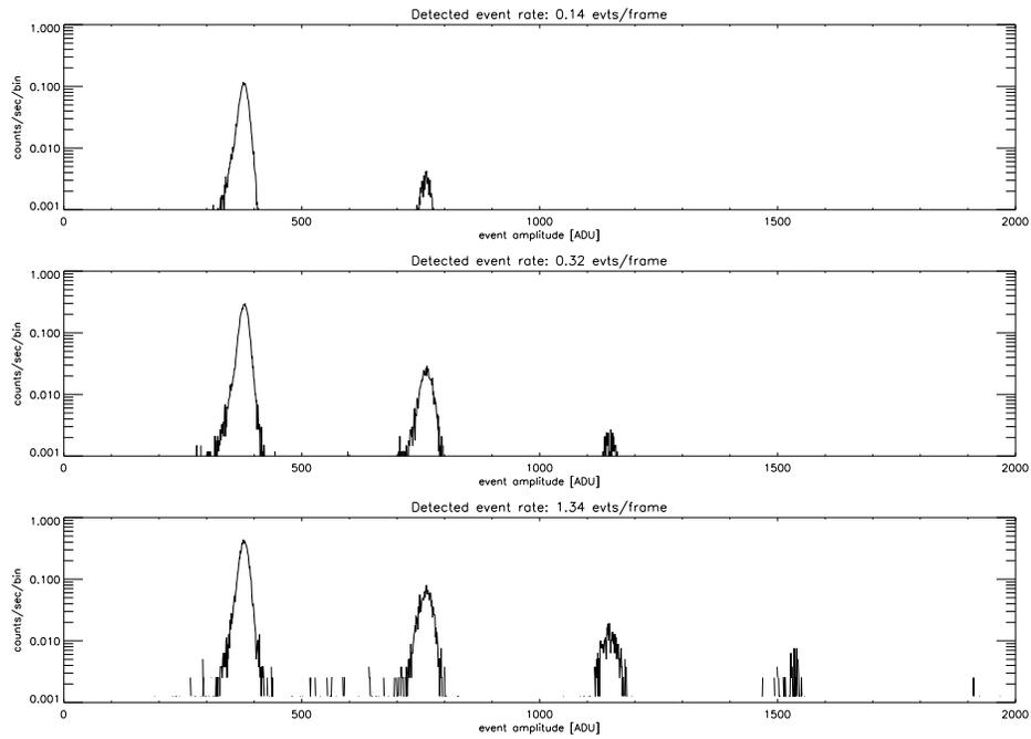
Figure 6.16: The effects of pileup at 1.49 keV ( $\text{Al K}\alpha$ ) as a function of source intensity. Data were taken during HRMA-ACIS system level calibration at the XRCF. Single-photon events are concentrated near the pulse height corresponding to the  $\text{Al K}\alpha$  line ( $\sim 380$  ADU), and events with 2 or more photons appear at integral multiples of the line energy.
