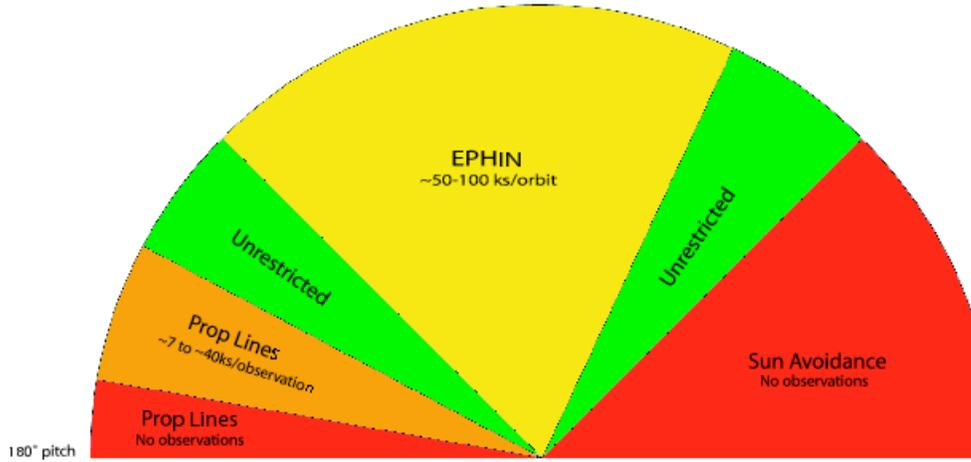
Figure 3.3: Diagram to illustrate ranges of solar pitch angle (the angle between the pointing direction and the satellite-Sun line) within which different observing limitations apply. Table 3.1 provides quantitative estimates for the observing limitations in the solar pitch angle ranges shown in the drawing.
