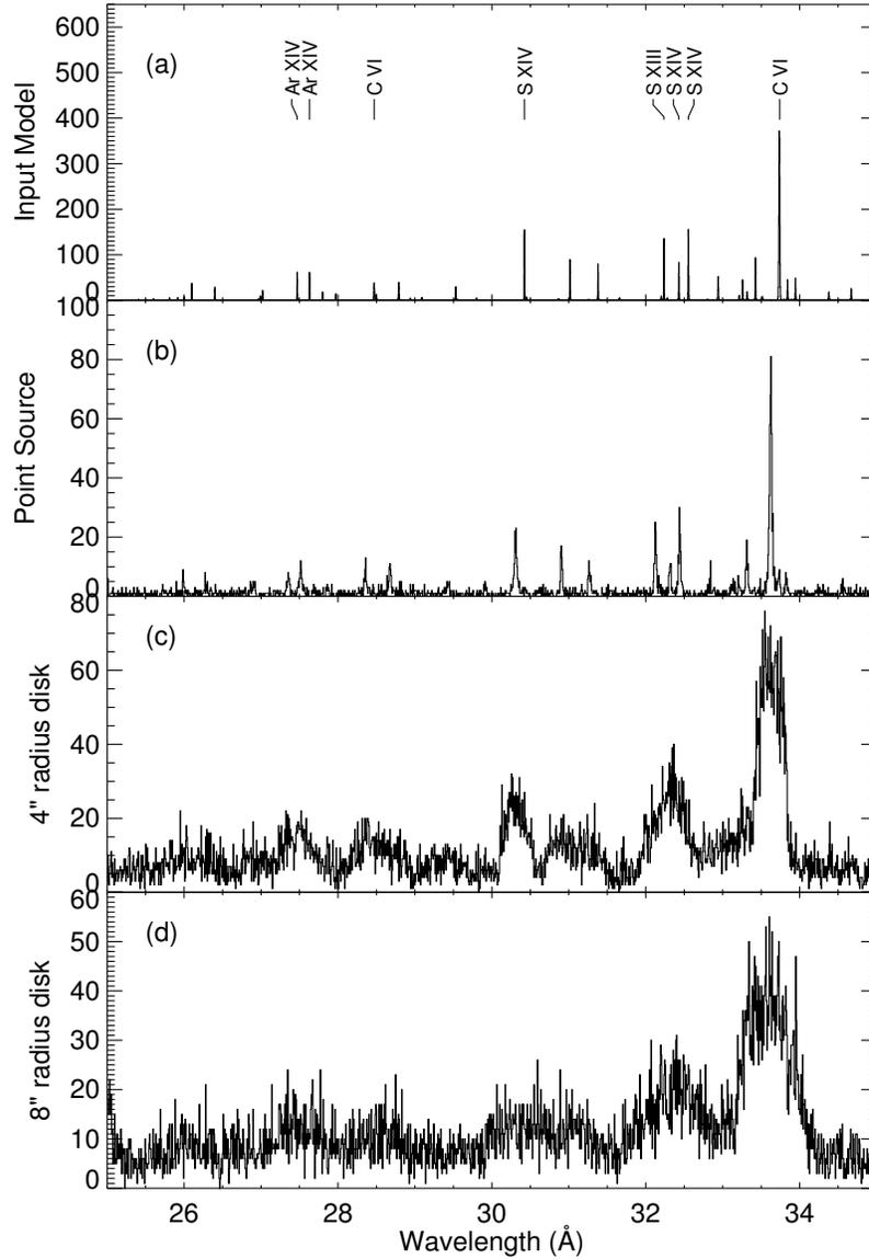
Figure 9.30: *MARX* simulation of spectra showing the effect of source extent. The panels show (a) computed input spectrum, (b) a *MARX* output of LETG spectrum of a point source, (c) the same as (b) except that the source is a disc of uniform brightness with radius of 4", and (d) the same but with radius of 8". See Figure 9.11 and Section 9.3.3 for a discussion of extended sources.
