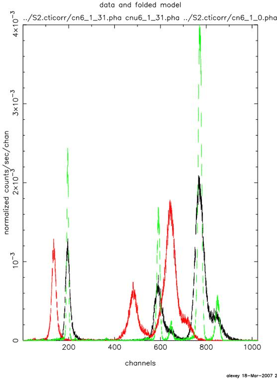
Fig. 1— The observed ECS spectra in the top (31st) segment of S2, node 1, Epoch 0, before (*red*) and after (*black*) the CTI correction. The spectra are extracted in the PHA space, binned by 2. For comparison, the green points show the spectrum observed near the readout (can be considered as an undamaged spectrum).
