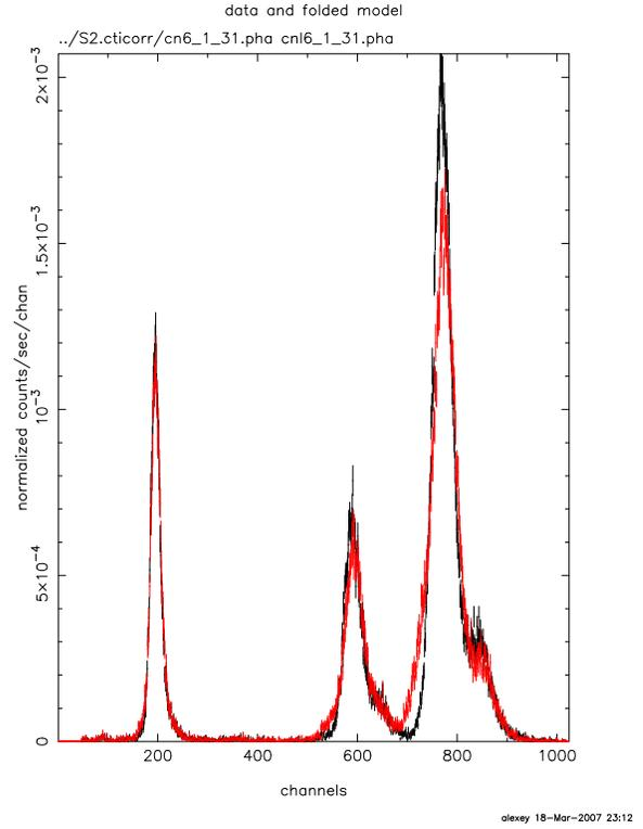
Fig. 2— Same as Fig.1 but the *red* points show the data corrected using the *light* algorithm.
