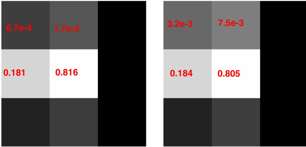
Fig. 3— Average image for the `fltgrade = 8`, Mn-K $\alpha$  events in the bottom *left* and top *right* 256 rows of S2. The images are normalized to a total flux of 1. The labels indicate the relative brightness of pixels.
