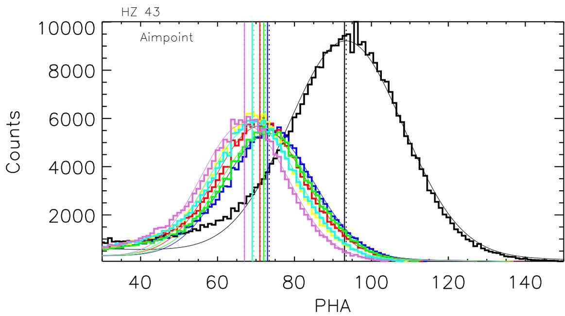
**Figure 4.** HZ 43 aimpoint PHA distribution. Solid vertical lines mark the median PHA. Gaussian fits over-plotted. Note: total counts vary in accordance with differing exposure times per observation.
