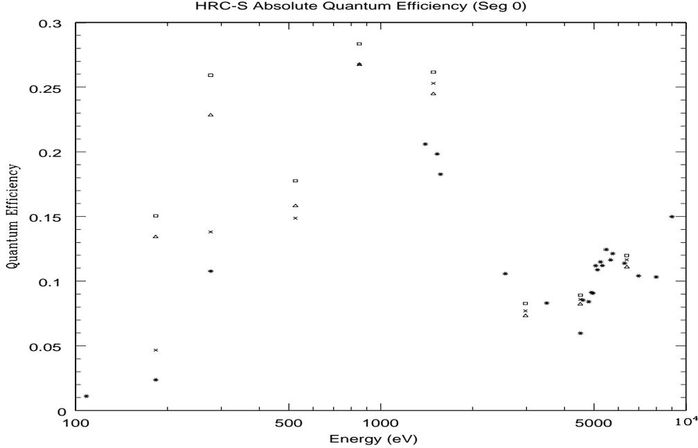
Figure 8: Absolute QE of HRC-S segment 0. The different symbols represent different regions of the detector: the cross is a central region under the thick Al, the open triangle and the open square are regions under the thin Al to the left (lower V coordinate) and right (higher V coordinate) of the central T region. The stars are the HRC-S QE derived from the XRCF data.
