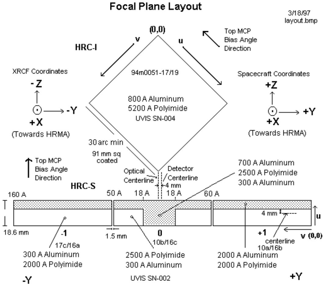
Figure 3: Schematic diagram of HRC UVIS and layout of the instrument.
