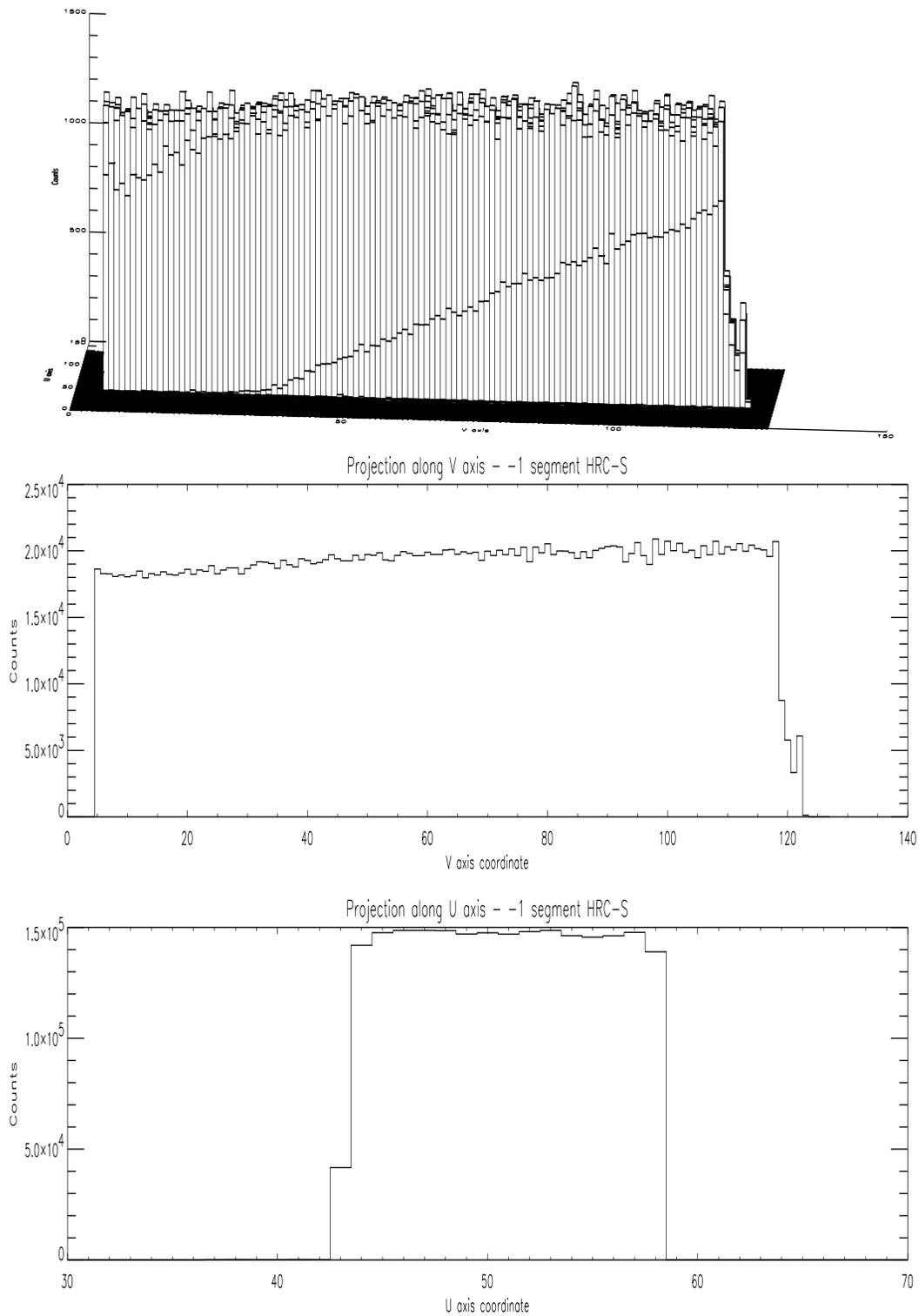
Figure 6: Surface plot and projections along the U and V axes of HRC-S segment -1, Al  $K_{\alpha}$ . Each pixel is 0.82 mm.
