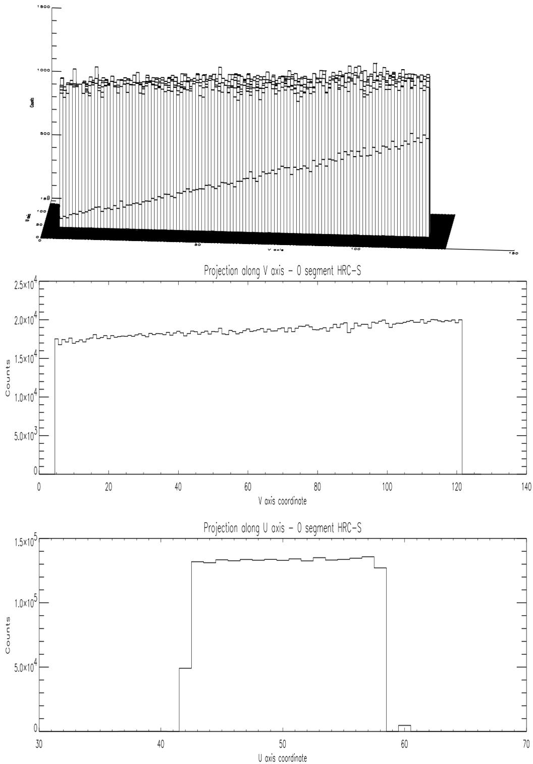
Figure 5: Surface plot and projections along the U and V axes of HRC-S segment 0, Al  $K_{\alpha}$ . Each pixel is 0.82 mm.
