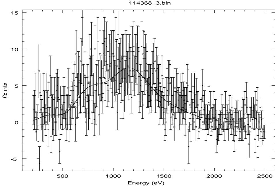
Figure 13: One BND-H spectrum of the HIREFS source (points) and best fit spectral model (histogram).
