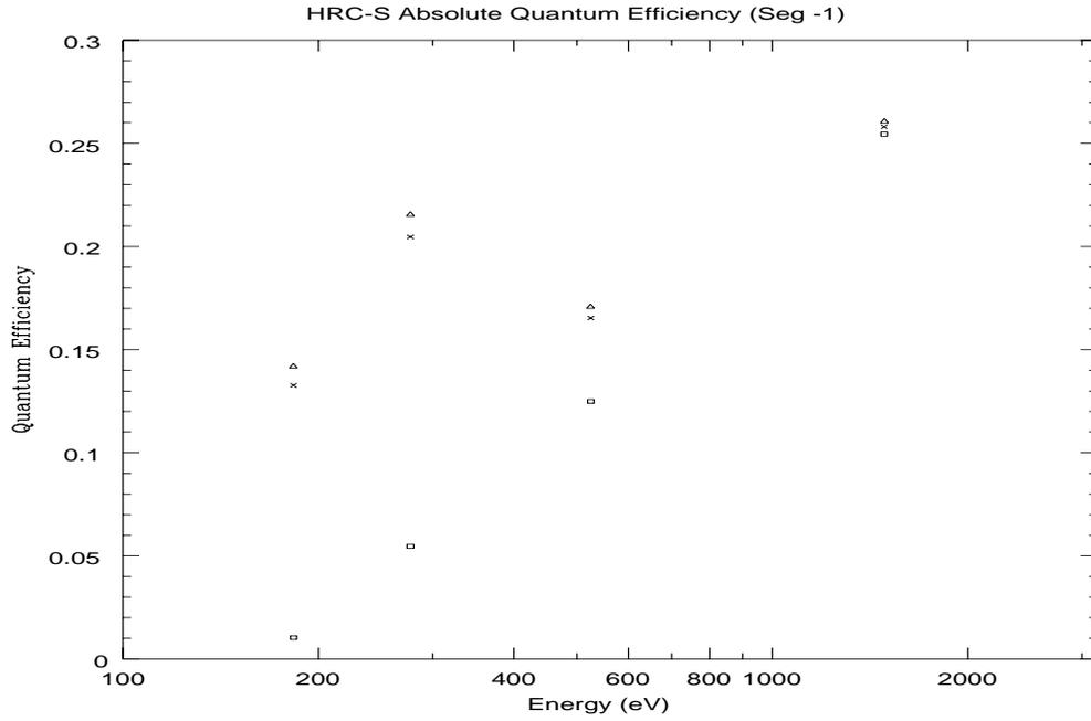
Figure 9: Absolute QE of HRC-S segment -1. The different symbols represent different regions of the detector: the open square is a region across the top under the thick Al, the cross and the open triangle are left (lower V coordinate) and right (higher V coordinate) regions under the thin Al.
