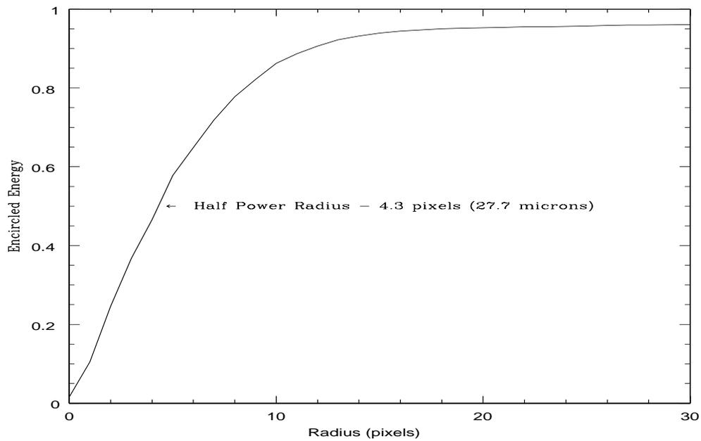
Figure 18: Encircled energy versus radius of the HRC-S/HRMA in focus at 277 eV.
