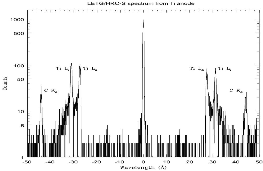
Figure 14: LETG/HRC-S spectrum of Ti anode with Ti filter. This plot is a projection of the HRC-S image along the dispersion direction.
