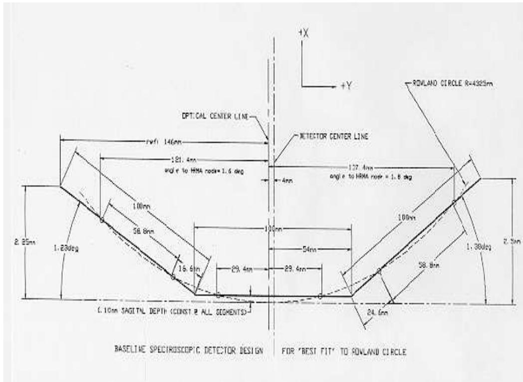
Figure 2: Schematic diagram of the layout of the three segments of the HRC-S. Note the tilt of the two wing segments relative to the center segment.
