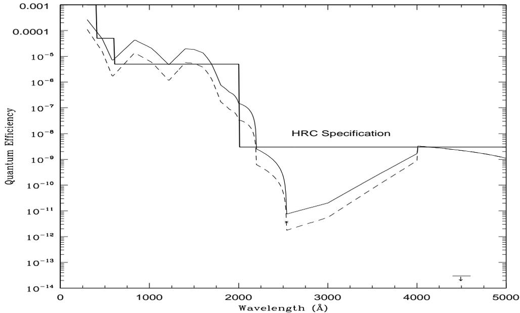
Figure 19: The calculated UV/optical QE of the wing segments of the HRC-S (the thin solid line) versus wavelength. The dashed line is the predicted QE for the nominal UVIS thickness plus the 2 sigma uncertainty. The measured values at 2537 Å and 4500 Å (an upper limit only) are also plotted. The dark solid line is the maximum UV/optical sensitivity specification. Note the logarithmic scale of the Quantum Efficiency axis.
