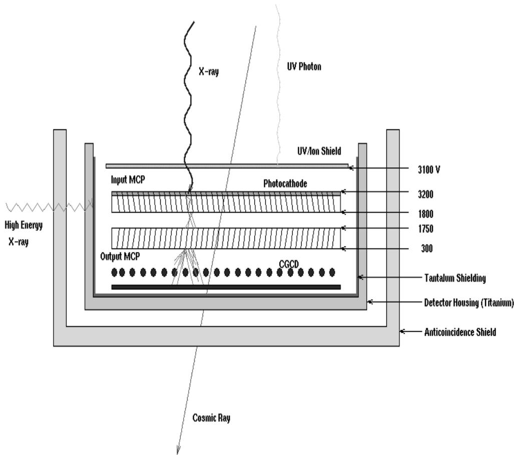
Figure 1: Functional diagram of the HRC showing the UVIS, MCPs, and modified CGCD. The tantalum shield and anti-coincidence shield are for background reduction/rejection.
