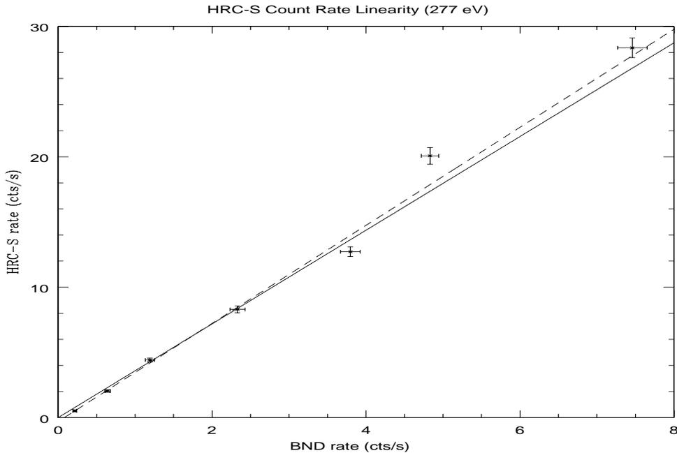
Figure 15: Count rate linearity of the HRC-S at 277 eV. The solid line is the best fit line if the fit is forced through the origin. The dashed line is the best fit line if the fit is not forced through the origin.
