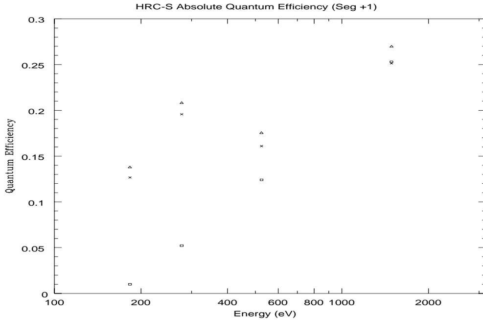
Figure 10: Absolute QE of HRC-S segment +1. The different symbols represent different regions of the detector: the open square is a region across the top under the thick Al, the cross and the open triangle are left (lower V coordinate) and right (higher V coordinate) regions under the thin Al.
