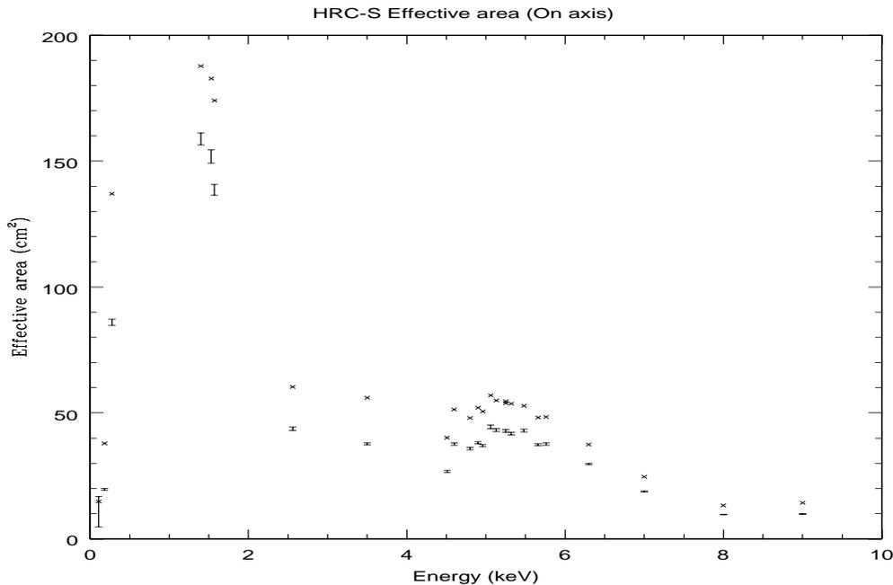
Figure 12: Effective area of the HRMA/HRC-S on axis
