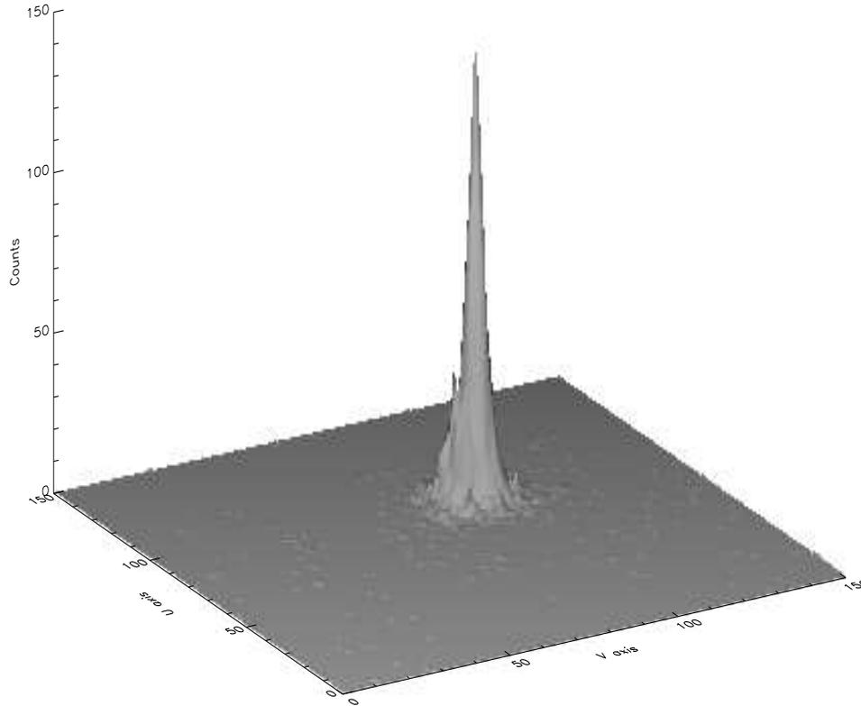
Figure 16: Point spread function of the HRC-S and HRMA
