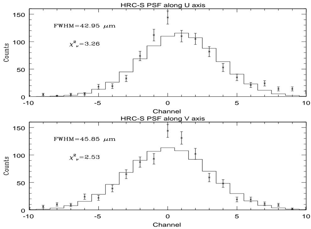
Figure 17: Best fit Gaussians to slices of the PSF along the U and V axes.
