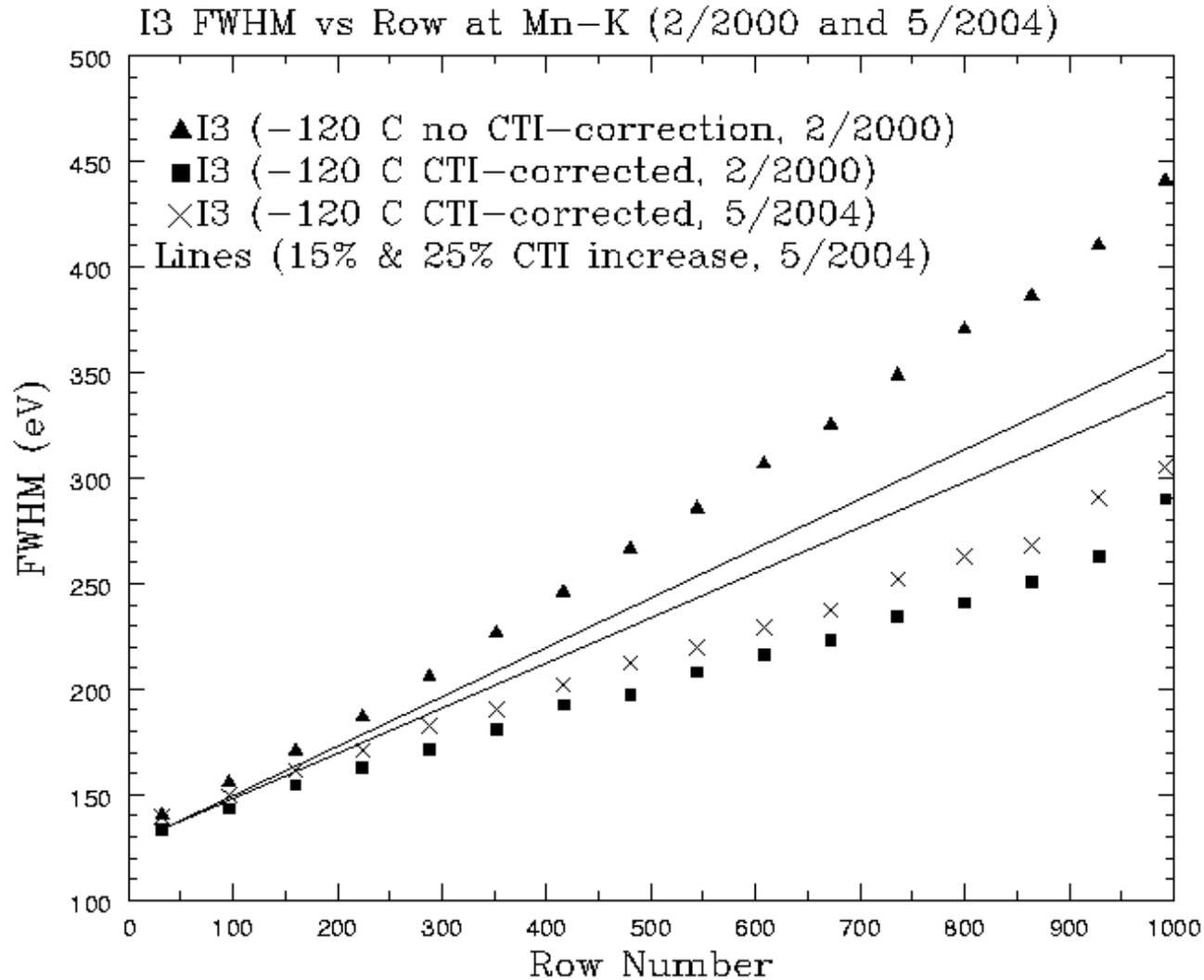
Predictions for FWHM include the 10% increase in CTI from 2000 to 2004 and the estimated 15.0% and 25.0% increase due to the bakeout.
