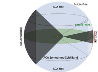
Heating and Cooling as a Function of Solar Pitch Angle
