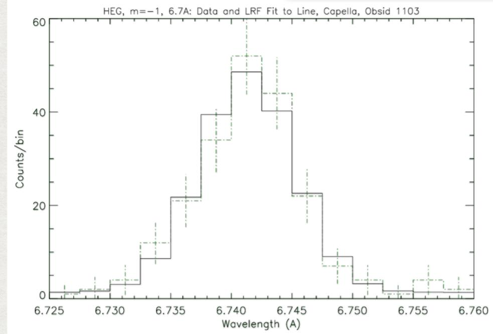
In-dispersion blur is the "Line Spread Function" due to both the imaging PSF and grating quality. Cross-dispersion is an imaging PSF (defocused). Both are included in the grating RMF.
