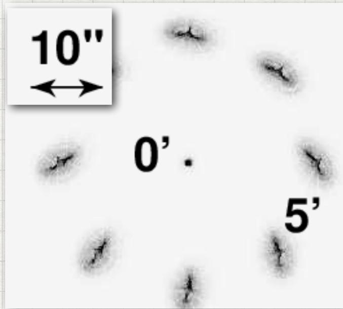
Simulated Mirror PSF vs. off-axis angle at 1.49 keV
