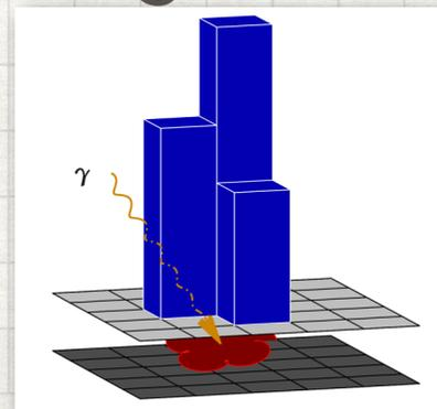
Detect photons with some efficiency vs energy (Quantum Efficiency, "QE"), but also detectors also interact with photons, and have "fuzzy" pixels. For CCDs, there is a "charge cloud" distributed over several pixels.
