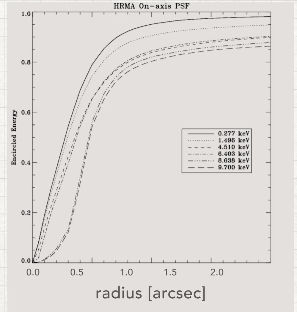
On-axis enclosed energy fraction vs energy.
