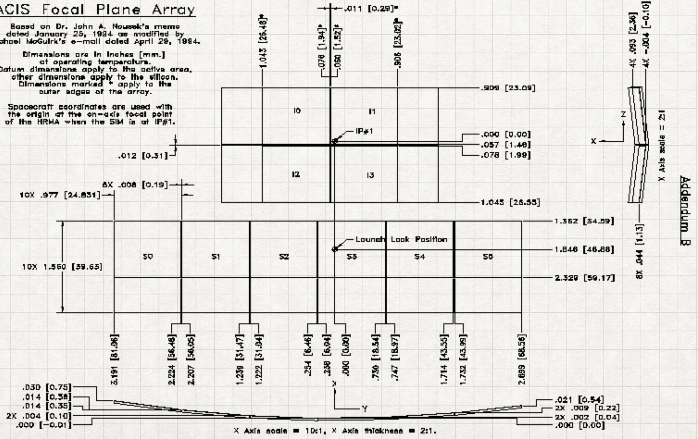
We need to accurately know the positions of all components so we can convert an event from a local detector coordinate to a focal plane 3D coordinate (relative to the mirror node), to an angle on the projected sky.
