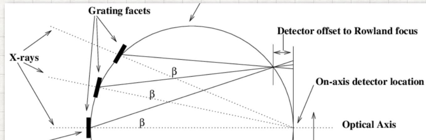
Change the angle according to energy, with some efficiency (vs. order), and with some scatter (Line Spread Function, "LSF")
