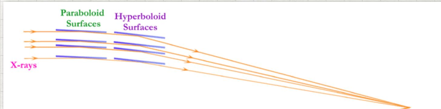
... and some fraction exit, over a distribution of angles (Point Spread Function, "PSF"). Efficiency and PSF depend on energy and angles.
