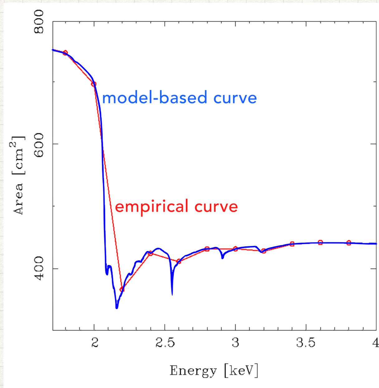
Calibration *must* be underpinned with physical models (reflectivity, diffraction efficiency, detector physics, transmission models).
