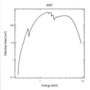
**Figure 2.** Effective area curve for chip 1 of the Chandra ACIS detector. The effective area varies as a function of energy, quite significantly. This variation must be included in a model fitted to a Chandra observation.
