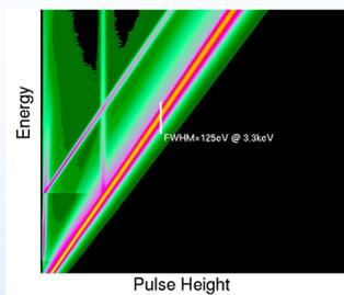
**Figure 3.** ACIS response matrix. The response matrix accounts for how the detector redistributes photons of a given energy. For photons of energy  $E$ , there is a probability distribution that describes how many counts can be expected in each detector channel. As this figure shows, the peak of the distribution shifts to greater pulse height amplitudes, or detector channel, as incoming photon energy increases.
