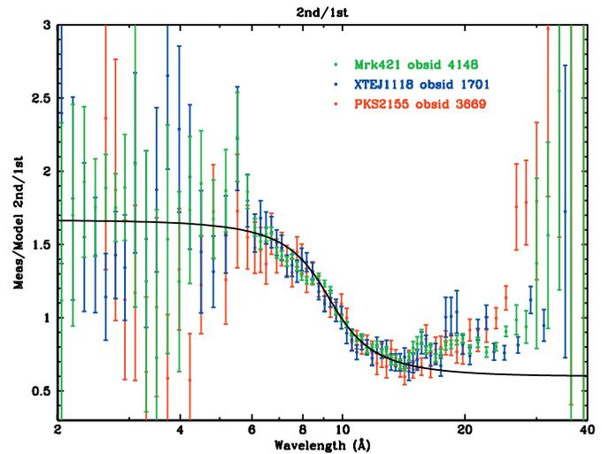
FIGURE 11: Comparison between measured and model ratios of 2nd/1st order LETG diffraction efficiencies (figure courtesy of Brad Wargelin).
