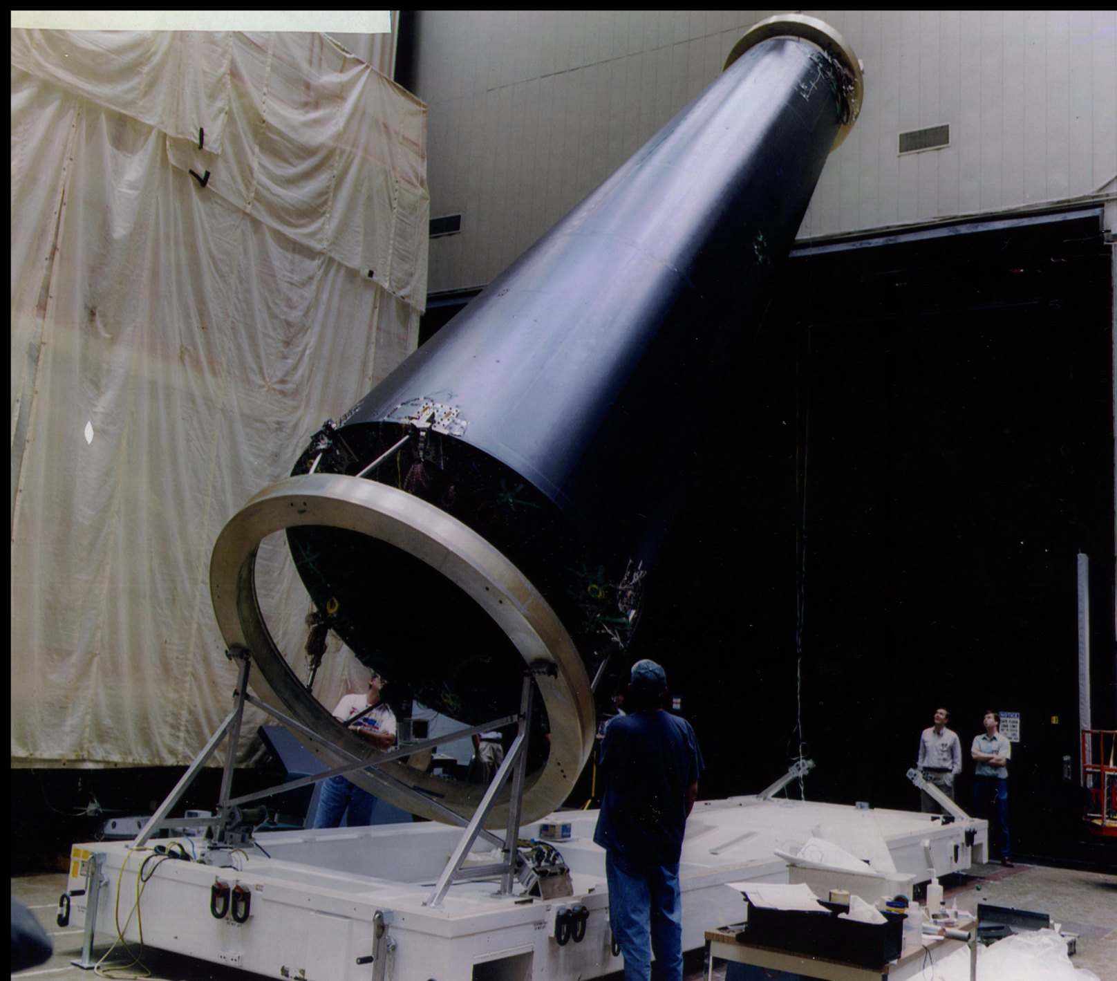
Structure being prepared for Static Load Test in Handling Fixture
