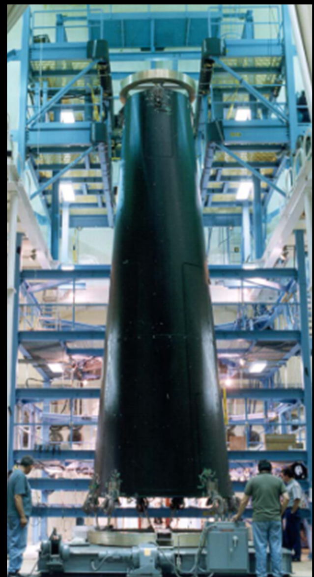
Completed OBA with blankets installed being prepared for HRMA integration at NGAS
