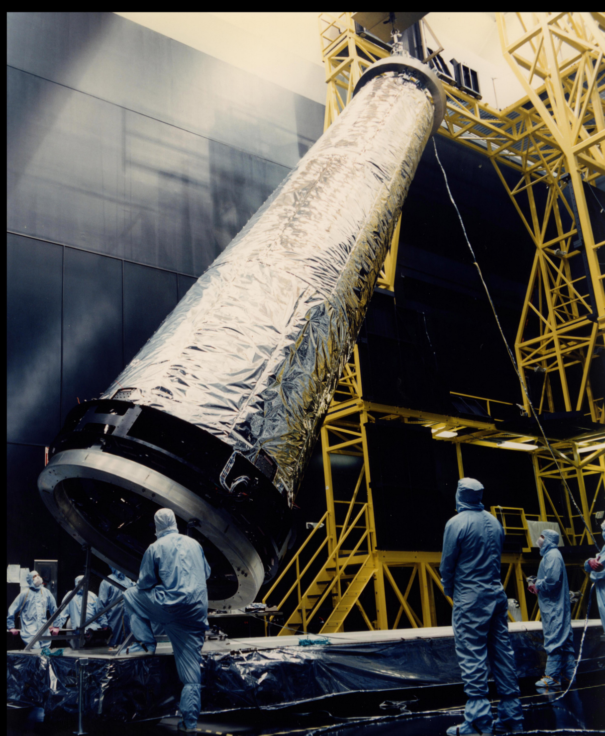
Completed OBA with blankets installed being prepared for HRMA integration at NGAS
